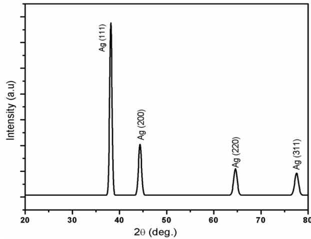
Fig. S2: XRD plot of the sample having film thickness value  $d = 185$  nm.
