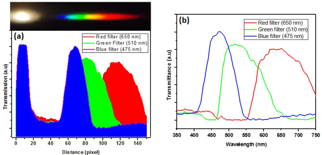
Fig. S3: (a) The diffraction image and corresponding line profile (transmittance versus pixel location), and (b) The calibrated line profile (transmittance versus wavelength).
