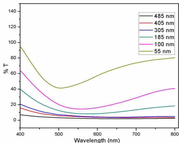
Fig. S4: The UV-visible transmittance spectra of Ag nanorods on DVD templates having different thickness values.
