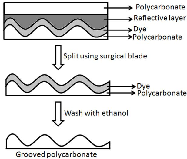
Fig. S1: Schematic showing the construction of grooved polycarbonate DVD grating substrate.
