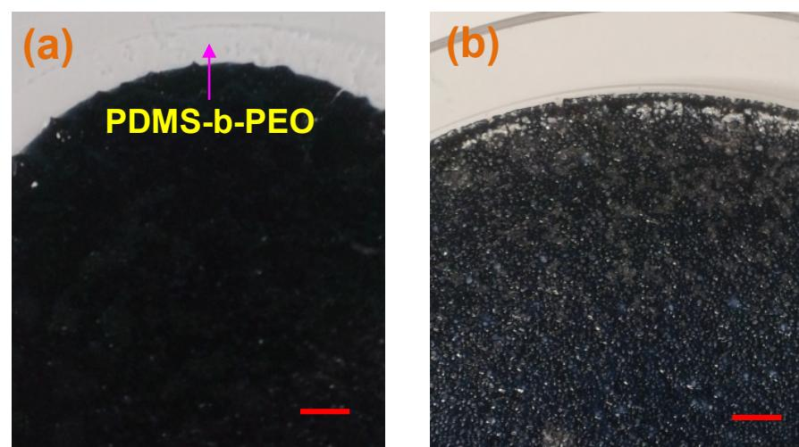
**Figure S1.** Photographs of polymer blend films consisting of (a) a 200% PEDOT:PSS, a 100% PDMS, and a 40% PDMS-b-PEO, and (b) a 300% PEDOT:PSS, a 100% PDMS, and a 30% PDMS-b-PEO, respectively. It is found from (a) that a PDMS-b-PEO phase is separated from the main blend film at this excess concentration of PDMS-b-PEO. (b) shows a higher concentration of PEDOT:PSS does not improve the film uniformity. Scale bars 5 mm.
