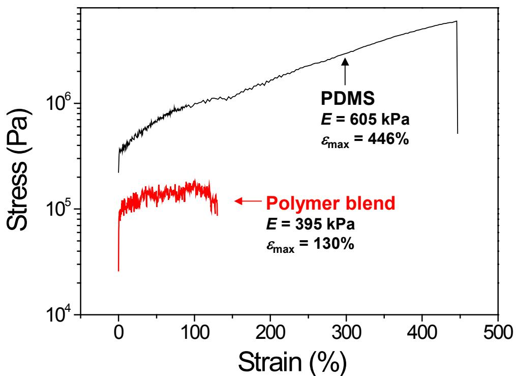
**Figure S5.** Tensile test results for a polymer blend film and a pure PDMS sheet. The composition of the blend film was same as that of a film with the largest rupturing strain ( $\sim 75\%$ ) in Fig. 5(c). Due to the incorporation of a large amount of PEDOT:PSS, which is mechanically weak, the mechanical properties of the blend film is deteriorated compared to pure PDMS sheet.
