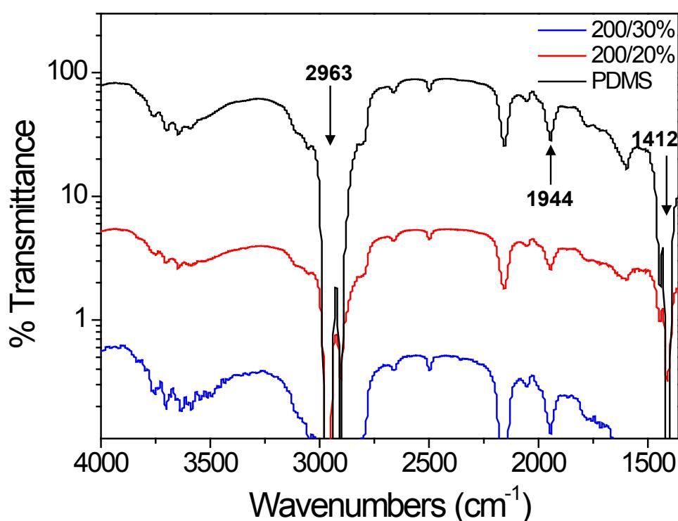
**Figure S2.** PEDOT:PSS:PDMS blend films show FT-IR profiles similar to that of a PDMS film, irrespective of the concentration of PDMS-b-PEO. This reflects that the blend films keep the main attributes of the PDMS film, thereby reinforcing their mechanical properties. The peaks at 2963 and 1412 cm<sup>-1</sup> correspond to CH stretching of CH<sub>3</sub> groups and CH<sub>3</sub> asymmetric deformation of Si-CH<sub>3</sub> bonds, respectively.
