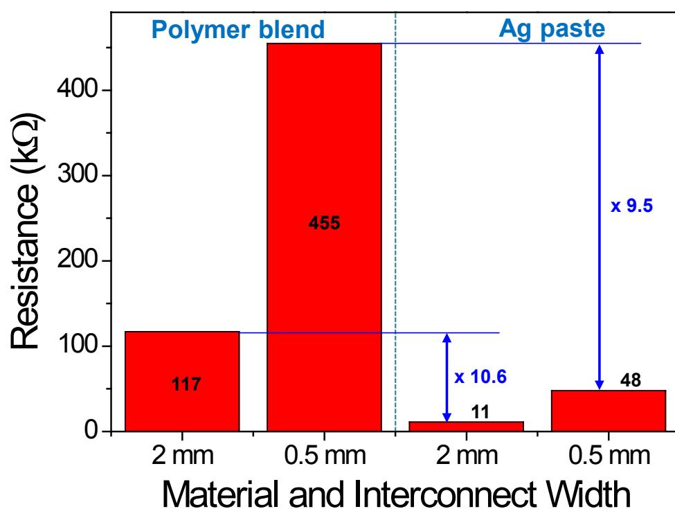
**Figure S6.** The resistance of a polymer blend interconnect appears to be about an order of magnitude higher than that of a control interconnect made of a Ag paste. This difference is originated from the conductivity difference of the two materials.
