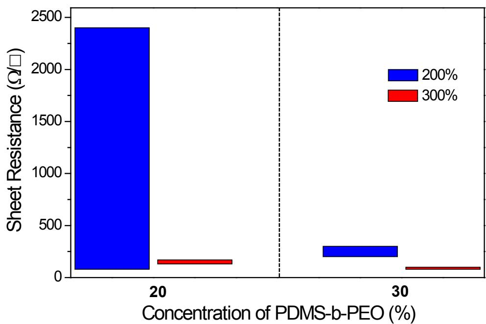
**Figure S4.** The sheet resistance of a polymer blend film is drastically reduced when the concentration of PEDOT:PSS increases. However, the increased PEDOT:PSS concentration is apt to weaken the mechanical property of the polymer blend as evidenced by Fig. 5(c), thus an optimal composition should be determined by a trade-off between electrical and mechanical properties.
