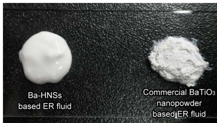
Fig. S6 Photograph of ER fluids based on 25 vol% of Ba-HNSs and commercial BaTiO 3 nanopowders.
