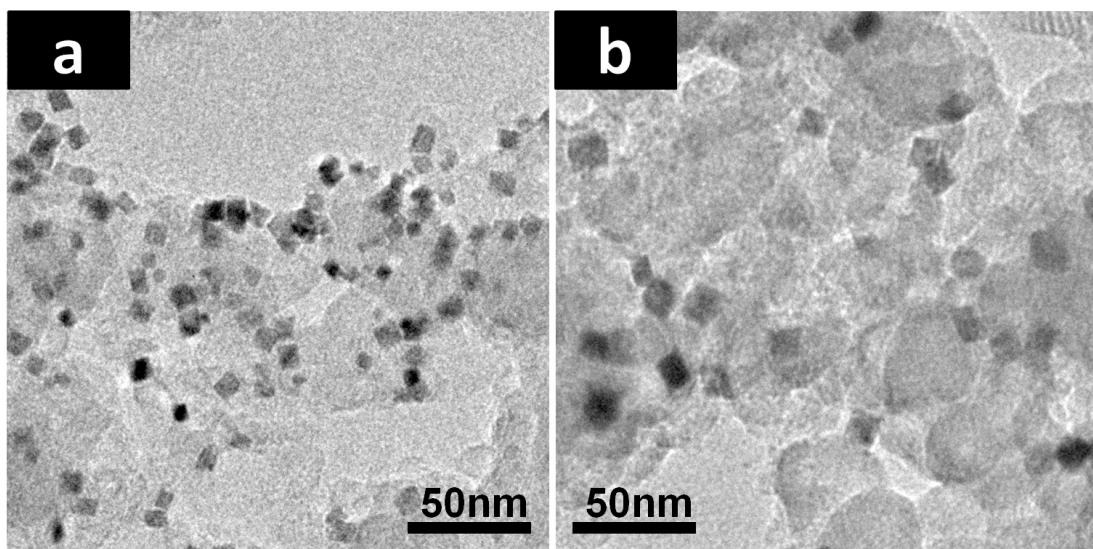
**Figure S9.** (a) 7nm and (b) 19nm octahedral  $\text{Pt}_3\text{Ni}$ -Fe NCs supported on carbon black.
