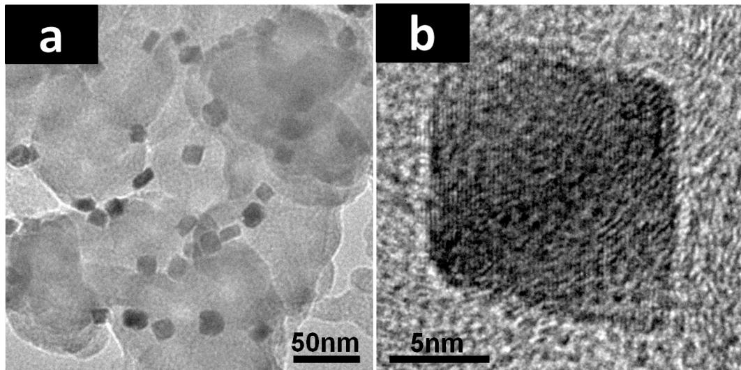
**Figure S11.** (a, b) 19nm octahedral NCs supported on carbon black after durability test.
