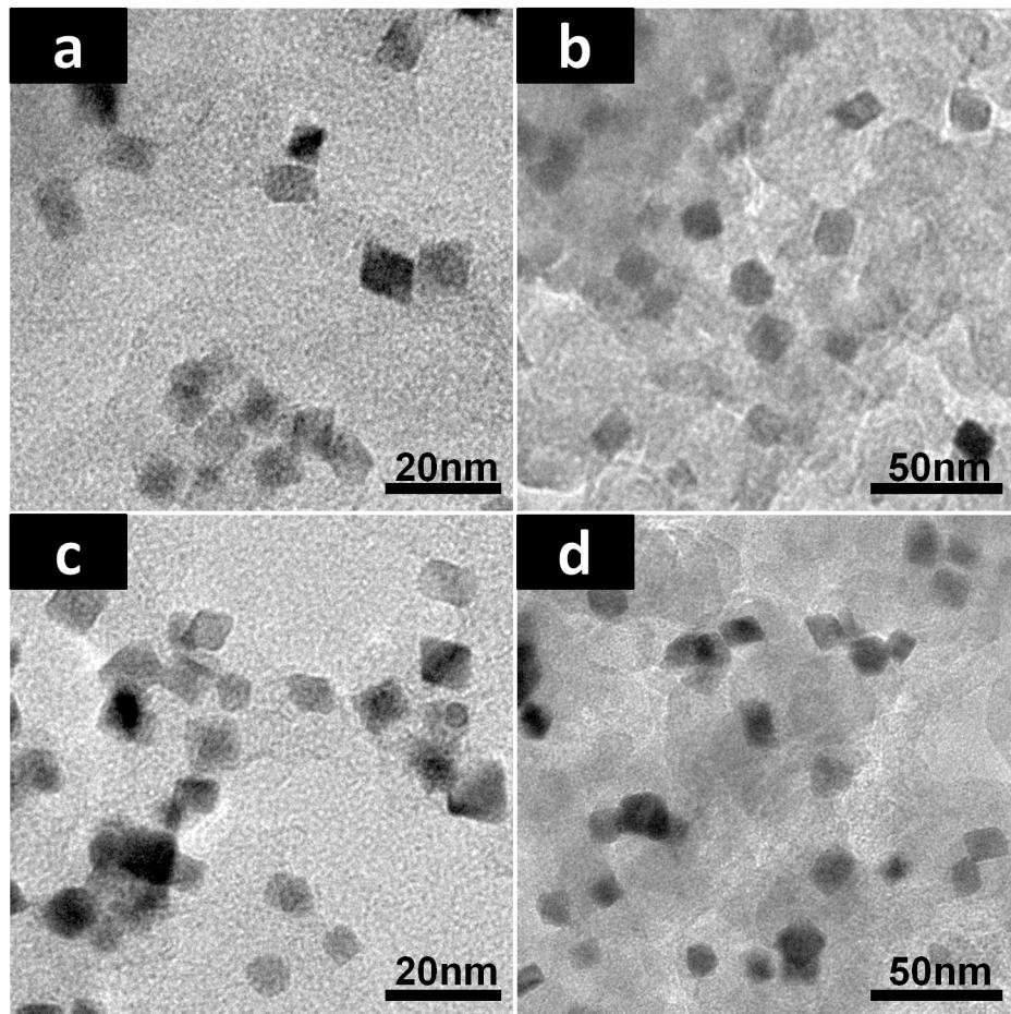
**Figure S5.** CB-supported octahedral NCs (a, b) before and (c, d) after thermal treatment.
