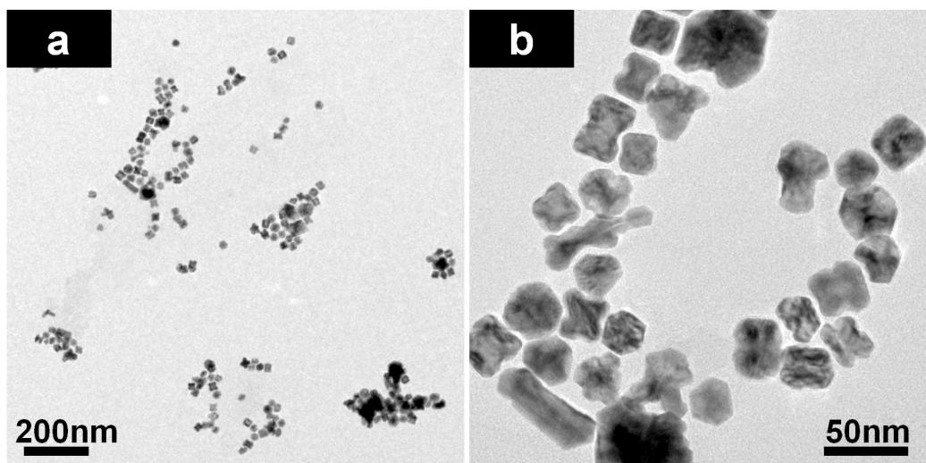
**Figure S1.**  $\text{Pt}_3\text{Ni}$ -Fe NCs synthesized with  $\text{Fe}(\text{acac})_2$  as the precursor of iron.
