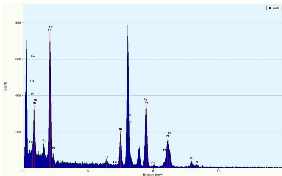
**Figure S2.** EDX spectrum of a single 7nm NC of  $\text{Pt}_3\text{Ni}$ -Fe.
