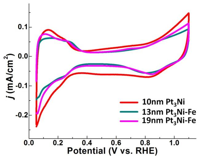
**Figure S6.** CV curves of 10nm  $\text{Pt}_3\text{Ni}$ , 13nm and 19nm  $\text{Pt}_3\text{Ni-Fe/C}$  electro-catalysts.
