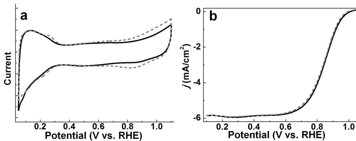
**Figure S10.** (a) CV and (b) LSV of 10nm octahedral  $\text{Pt}_3\text{Ni}/\text{C}$  catalysts before and after the durability test. (Solid black curve: Initial curve. Dashed grey curve: Final curve after durability test.)
