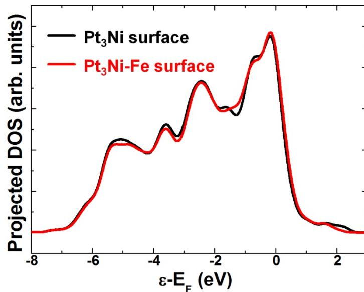
**Figure S8.** Density of states (DOS) of d-band for  $\text{Pt}_3\text{Ni}$  surface (black) and  $\text{Pt}_3\text{Ni}$ -Fe surface (red).
