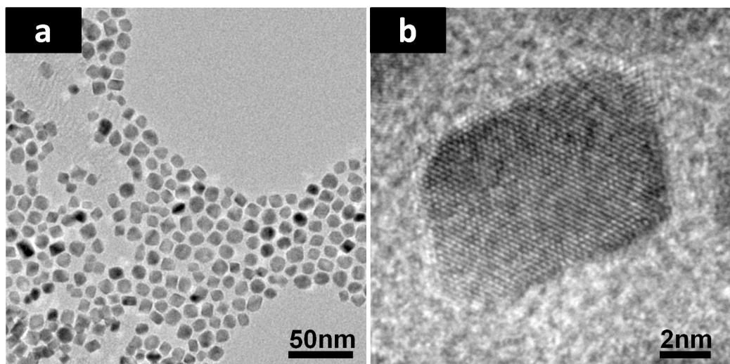
**Figure S3.** (a). TEM and (b). HRTEM images of 10nm octahedral  $\text{Pt}_3\text{Ni}$  NCs without the Fe doping.
