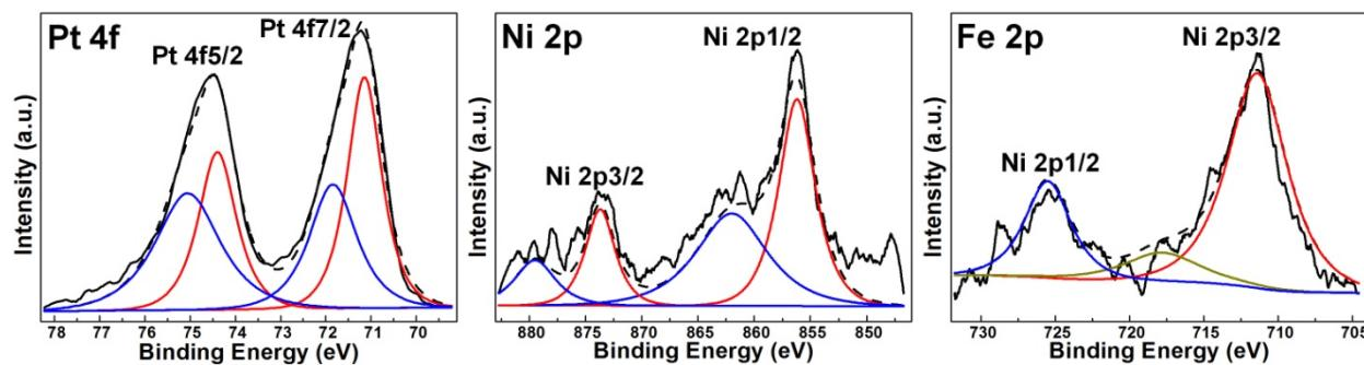
**Figure S7.** XPS spectra of Pt 4f, Ni 2p and Fe 2p regions for 7nm octahedral  $\text{Pt}_3\text{Ni}$ -Fe NCs.
