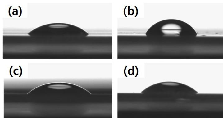
**Fig. S1** Water contact angle of (a) bare SiOx substrate(40.4°), (b) SiOx substrate after printing with a flat PDMS mold during 10min at 130°C(62.3°), (c) SiOx substrate after printing with air plasma-treated PDMS mold during 10min at 130°C(41°) and (d) SiOx substrate after printing with air plasma-treated PDMS mold during 10min at room temperature(42°).
