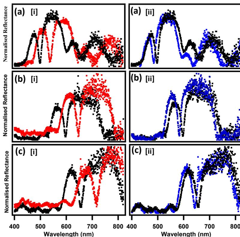
**Supl. Fig 7:** Normalised reflection spectra of PS Microcavities fabricated for different cavity resonances, (a) 493nm (b) 596nm and (c) 657 nm ( black colour curves), compared with [i] corresponding reflection spectra (Red colour) during short time exposure to methanol (reversible) and [ii] corresponding recovered reflection spectra ( blue color) after prolonged exposure and dried PS cavities ( semi-permanent). See mail text for further information.
