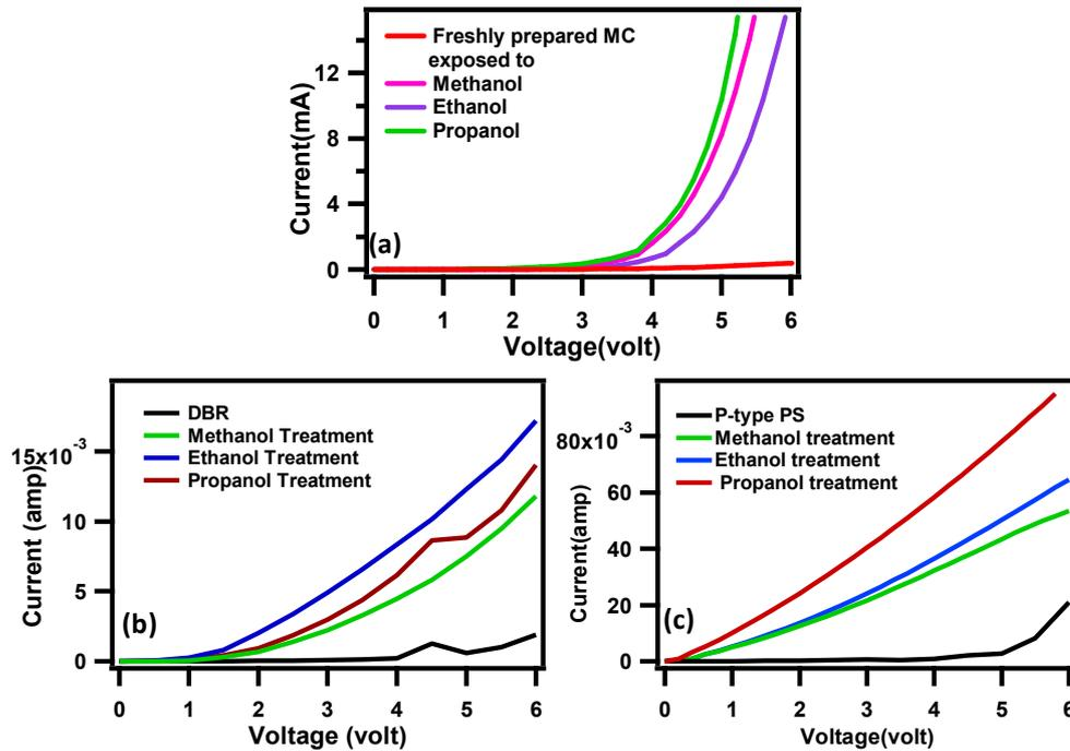
**Sup. Fig. 3** Current-voltage measurement of (a) Microcavity (b) DBR, (c) p-type single layer. It is found that there is a different amount of current enhancement corresponding to different Solvent having different dielectric constant for all the photonic structures such as MC, DBR, p-type single layer.
