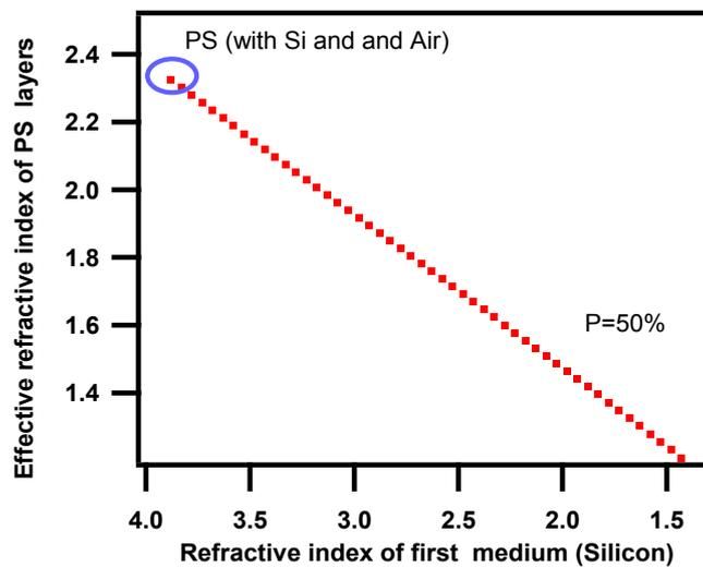
**Sup. Fig 6** Simulated effective refractive index of single PS (p=50%) layer with an assumption that the 1<sup>st</sup> medium silicon ( $n_{si}= 3.6$ ) is functionalised by unknown chemical species ( see text). Here the refractive index of 2<sup>nd</sup> medium ( $n_{air}=1.0$ ) and porosity/thickness remain constant. This is to support the experimental details related to figure 5.
