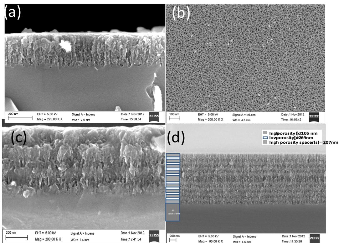
**Sup. Fig.1.** Example SEM pictures of (a) single porous layer cross-section and (b) top view (70% porosity), (c) Distributed Bragg Reflector (DBR) contains 8 layers of alternative porosities ( $n_1$  and  $n_2$ ) and (d) microcavity contains a spacer layer sandwiched between two DBRs.
