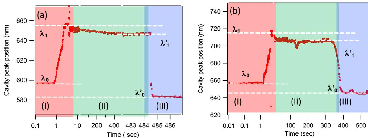
**Supl. Fig 6:** PS Microcavity resonant peak dynamic variation during solvent (methanol) exposure ( similar to Fig 5) for PS cavities of cavity resonances (a) 596nm and (b) 657nm. ( see Fig 5 and related text for further information)
