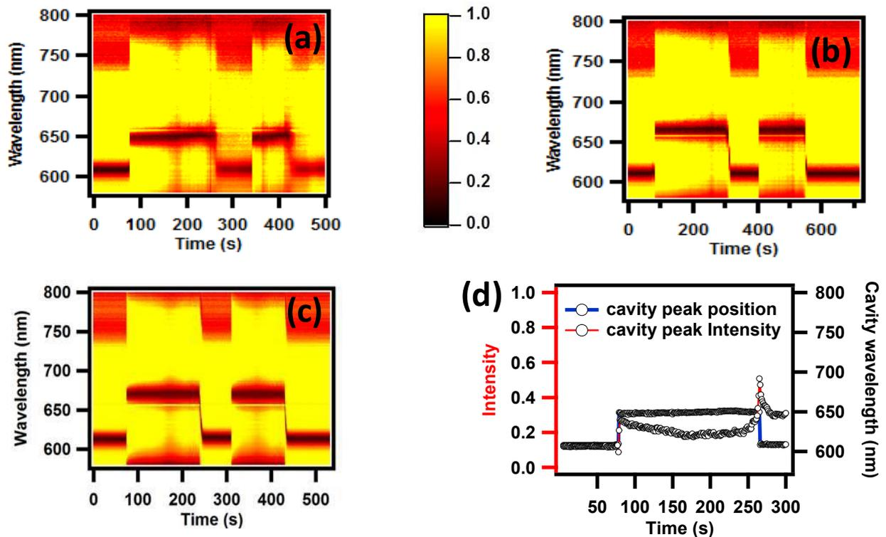
**Sup. Fig. 4** Reflection spectral mapping of microcavity on various short-time exposures of (a) Methanol (b) Ethanol (c) Propanol. Figure (d) shows the extracted cavity peak ( $\sim 613$ nm) variation (blue) and intensity (red) from Fig (a). The cavity resonances for shorter duration are consistently reversible for repeated exposure cycles.
