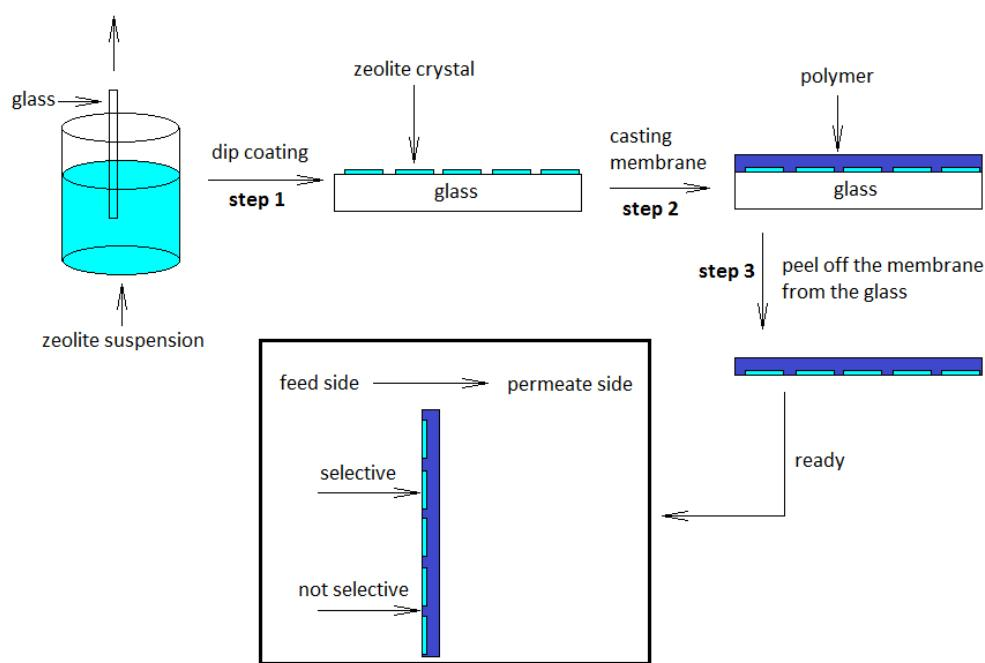
Fig S1. Preparation of surface sieving membrane.
