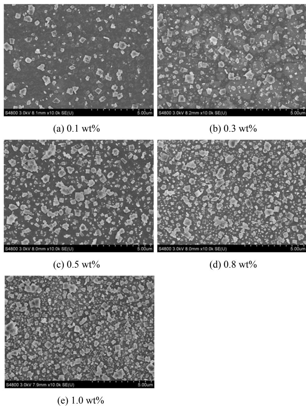
Fig S3. SEM images glass substrates dip coated in SAPO-34 suspensions with different concentrations.
