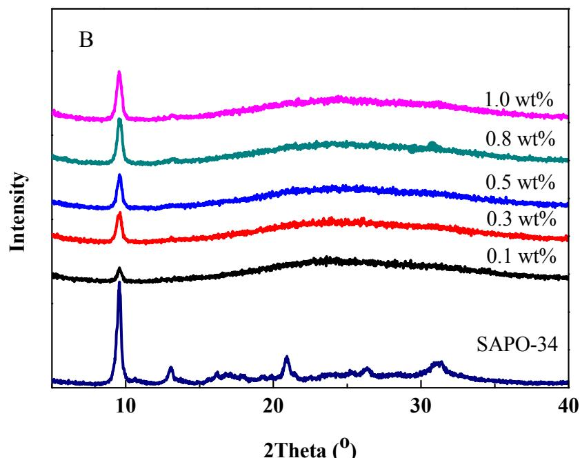
Fig S2. XRD patterns of glass substrates dip coated in SAPO-34 suspensions with different concentrations.
