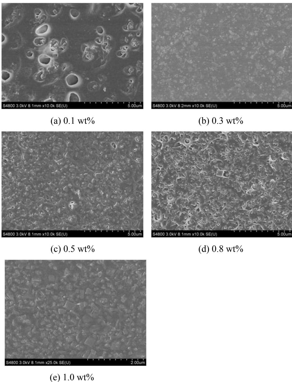
Fig S5. Top view SEM images of surface sieving membranes prepared with different SAPO-34 loadings.
