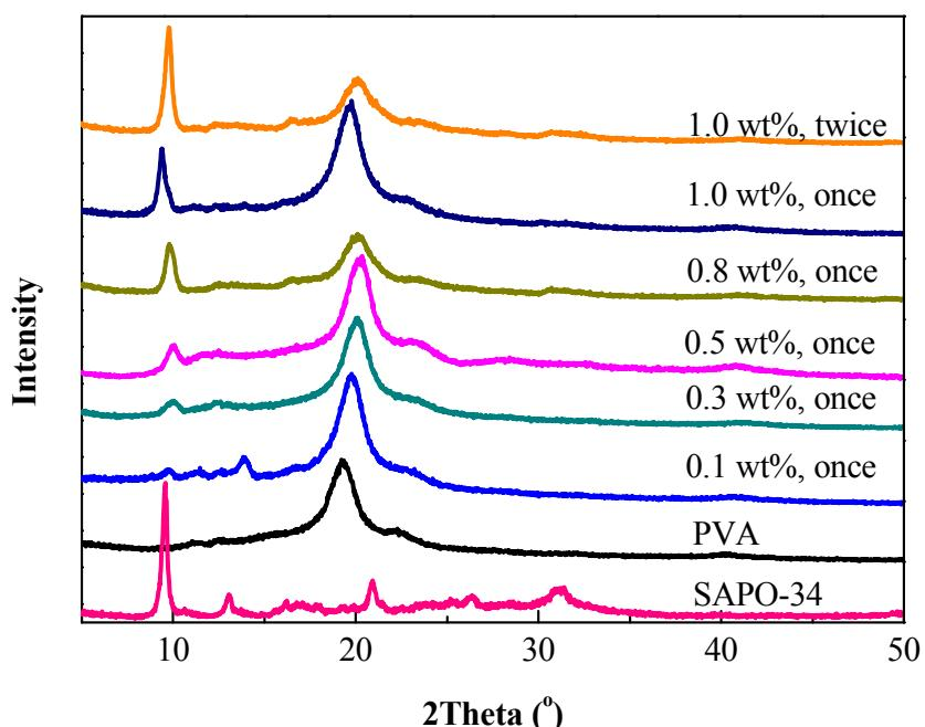
Fig S4. XRD patterns of surface sieving membranes prepared with different SAPO-34 loadings.
