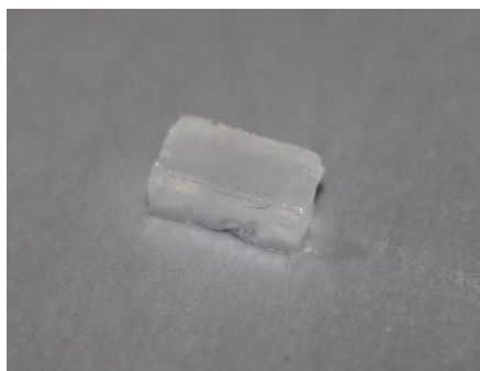
Figure S1. The image of silica gel which was fabricated at the concentration of 15% and cut into cube.
