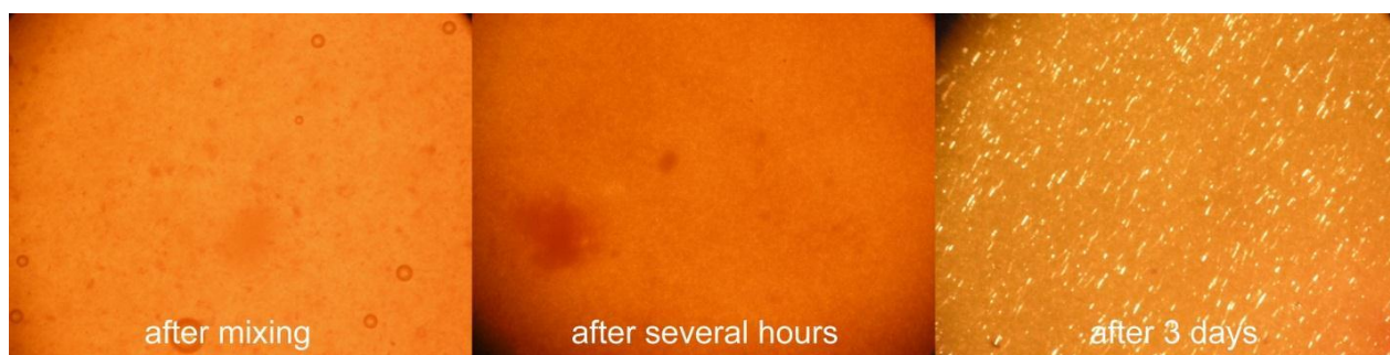
Figure S1. Effect of aging films of NaCas doped with PHA during the preparation. Left: the appearance of the solution immediately after mixing of the NaCas and PHA solutions. Middle: The same solution after several hours. Right: The film obtained after 3 days. Crystals reflect white light from their surface.
