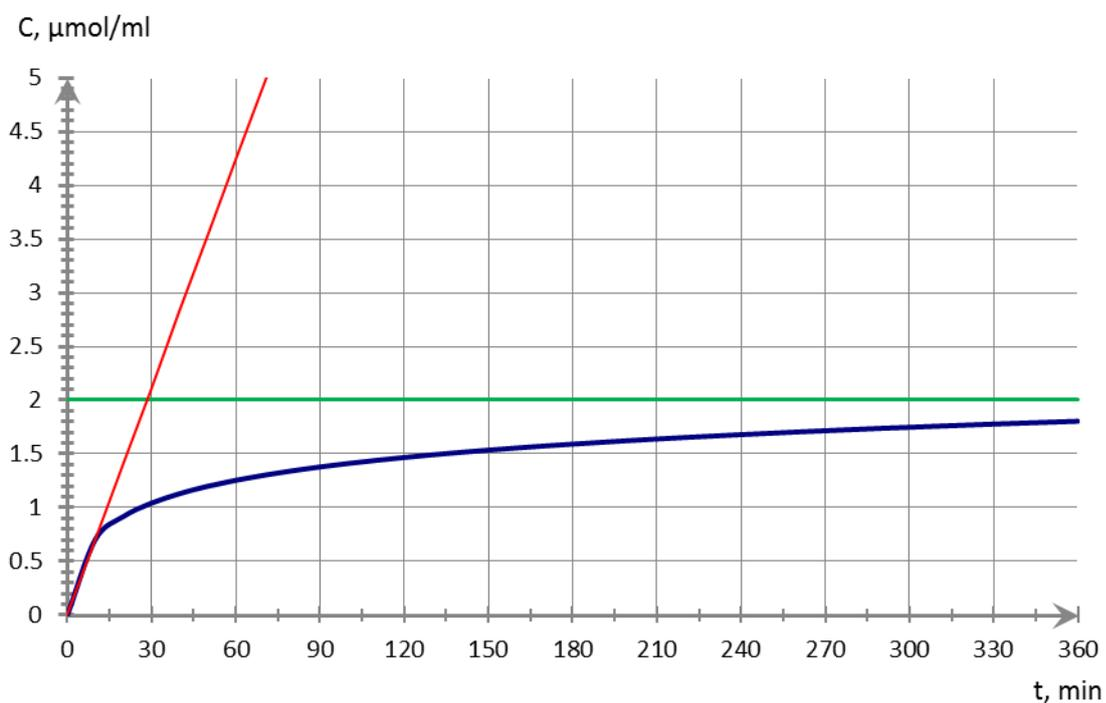
**Figure S20.** Initial rate of the exchange process between  $[(p\text{-cymene})_4\text{Ru}_4(5,8\text{-dioxydo-1,4-naphthoquinonato})_2(\text{bpy-}H_8)_2]^{4+}$  and  $\text{bpy-}D_8$  at 40°C with a 1:1 ratio.
