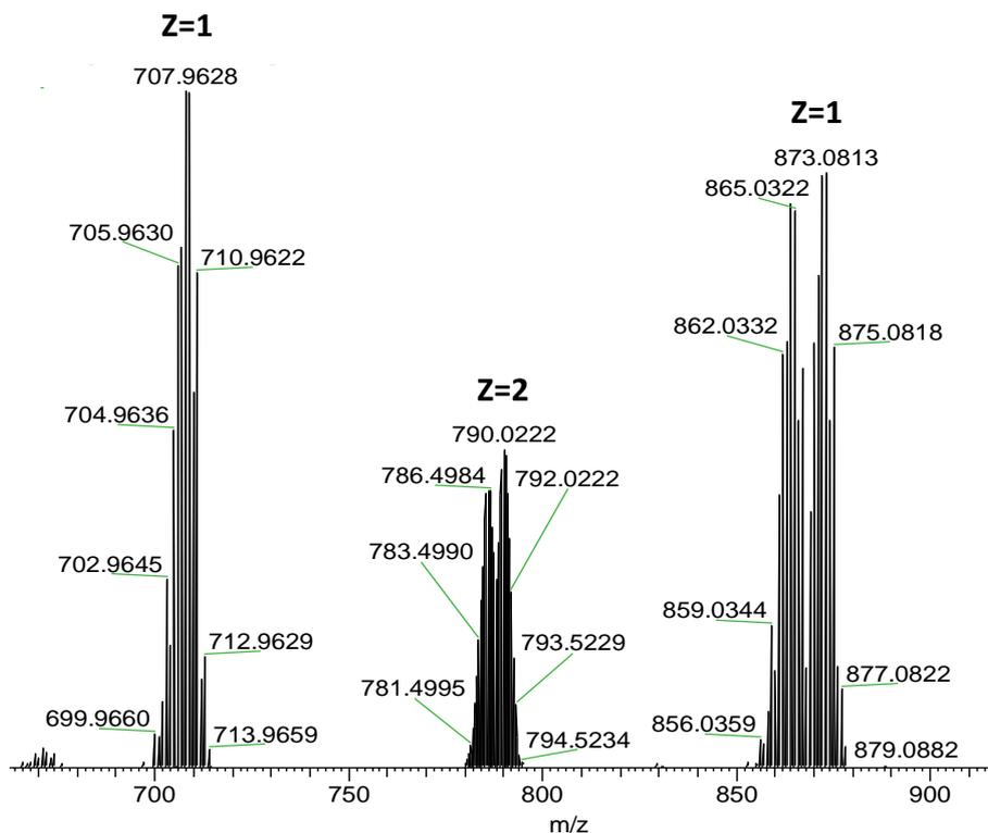
**Figure S1.** ESI-MS spectrum of  $[(p\text{-cymene})_4\text{Ru}_4(\text{oxalato})_2(\text{bpy})_2](\text{CF}_3\text{SO}_3)_4$  after mixing the two homo-rectangles ( $t = 0\text{h}$ ).
