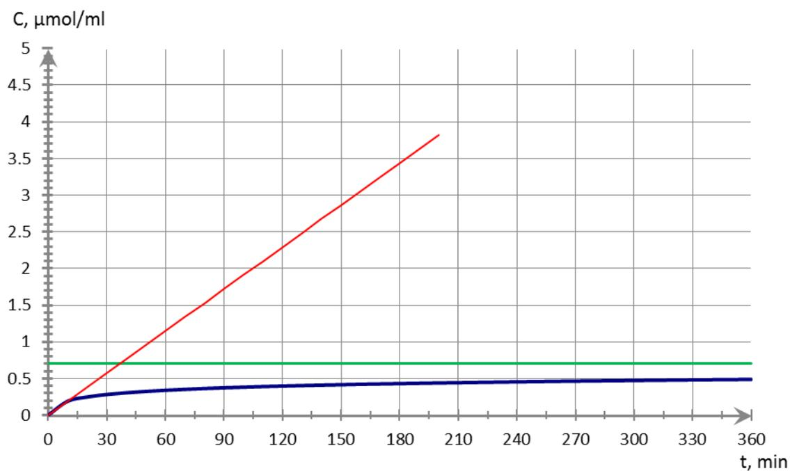
**Figure S17.** Initial rate of the exchange process between  $[(p\text{-cymene})_4\text{Ru}_4(2,5\text{-dioxydo-1,4-benzoquinonato})_2(\text{bpy-}H_8)_2]^{4+}$  and  $\text{bpy-}D_8$  at  $40^\circ\text{C}$  with a 1:1 ratio.
