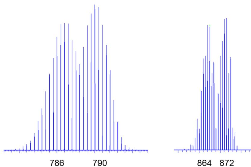
**Figure S8.** ESI-MS peaks corresponding to the species  $[(p\text{-cymene})_4\text{Ru}_4(\text{oxalato})_2(\text{bpy}) + 2\text{CF}_3\text{SO}_3]^{2+}$  and  $[(p\text{-cymene})_2\text{Ru}_2(\text{oxalato})(\text{bpy}) + \text{CF}_3\text{SO}_3]^+$  (right).
