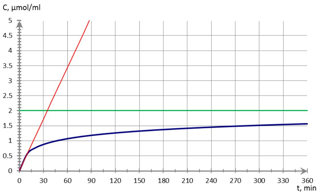
**Figure S11.** Initial rate of the exchange process between  $[(p\text{-cymene})_4\text{Ru}_4(\text{oxalato})_2(\text{bpy-}H_8)_2]^{4+}$  and  $\text{bpy-}D_8$  at room temperature with a 1:1 ratio.
