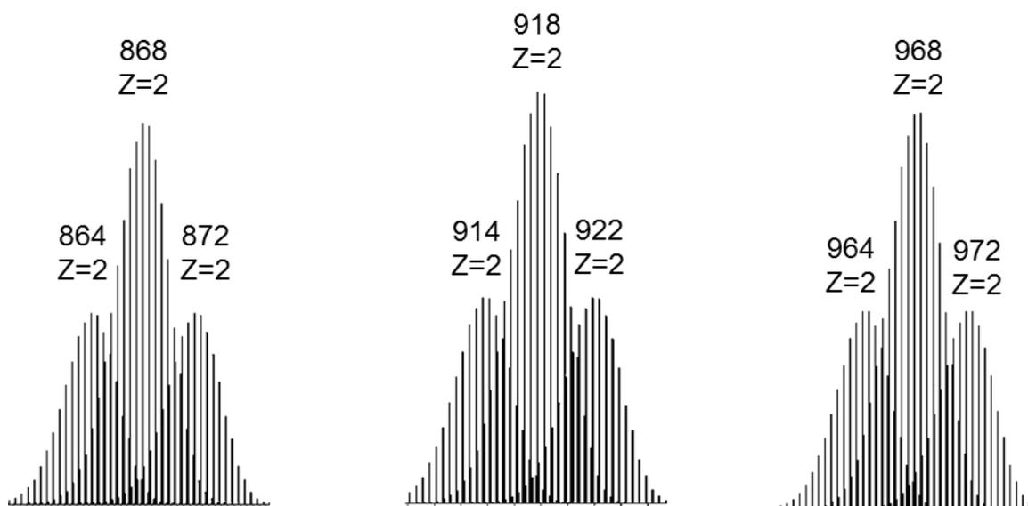
**Figure S6.** Calculated ESI-MS peaks corresponding to the species (in a 1:2:1 ratio),  $[(p\text{-cymene})_4\text{Ru}_4(\text{oxalato})_2(\text{bpy})_2 + 2 \text{CF}_3\text{SO}_3]^{2+}$  (left),  $[(p\text{-cymene})_4\text{Ru}_4(2,5\text{-dioxydo-1,4-benzoquinonato})_2(\text{bpy})_2 + 2 \text{CF}_3\text{SO}_3]^{2+}$  (middle) and  $[(p\text{-cymene})_4\text{Ru}_4(5,8\text{-dioxydo-1,4-naphthoquinonato})_2(\text{bpy})_2 + 2 \text{CF}_3\text{SO}_3]^{2+}$  (right).
