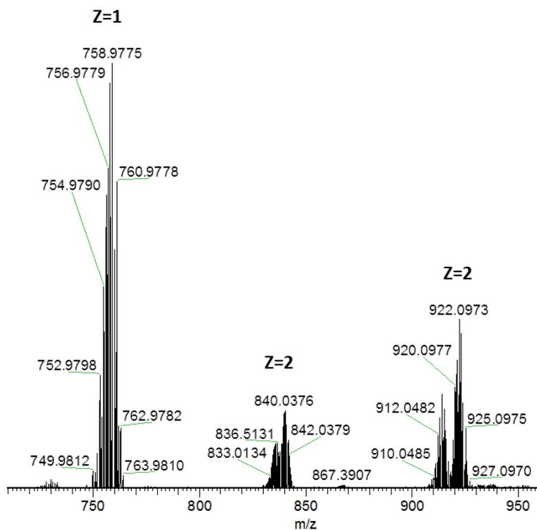
**Figure S2.** ESI-MS spectrum of  $[(p\text{-cymene})_4\text{Ru}_4(2,5\text{-dioxydo-1,4-benzoquinato})_2(\text{bpy})_2](\text{CF}_3\text{SO}_3)_4$  after mixing the two homo-rectangles ( $t = 0\text{h}$ ).
