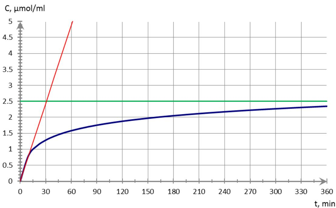
**Figure S19.** Initial rate of the exchange process between  $[(p\text{-cymene})_4\text{Ru}_4(5,8\text{-dioxydo-1,4-naphthoquinonato})_2(\text{bpy-}H_8)_2]^{4+}$  and  $\text{bpy-}D_8$  at room temperature with a 1:10 ratio.
