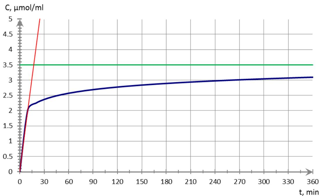
**Figure S13.** Initial rate of the exchange process between  $[(p\text{-cymene})_4\text{Ru}_4(\text{oxalato})_2(\text{bpy-}H_8)_2]^{4+}$  and  $\text{bpy-}D_8$  at  $40^\circ\text{C}$  with a 1:1 ratio.
