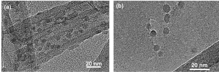
**Fig. S2** TEM images of MnFe<sub>2</sub>O<sub>4</sub>/halloysite nanocomposites (HF-2) with ferrite nanoparticles located the outer surface of halloysite nanotubes.
