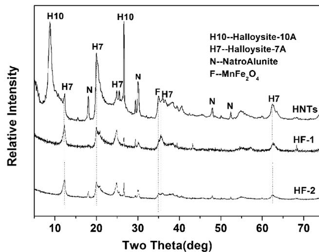
**Fig. S1** XRD patterns of natural halloysite (HNTs), MnFe<sub>2</sub>O<sub>4</sub>/halloysite nanotubular encapsulates (HF-1), and MnFe<sub>2</sub>O<sub>4</sub>/halloysite nanocomposites (HF-2).
