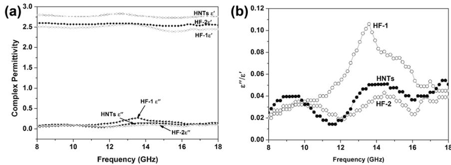
**Fig. S3** Frequency dependence of (a) relative complex permittivity, and (b) dielectric loss tangents of natural halloysite (HNTs), MnFe<sub>2</sub>O<sub>4</sub>/halloysite nanotubular encapsulates (HF-1), and MnFe<sub>2</sub>O<sub>4</sub>/halloysite nanocomposites (HF-2).
