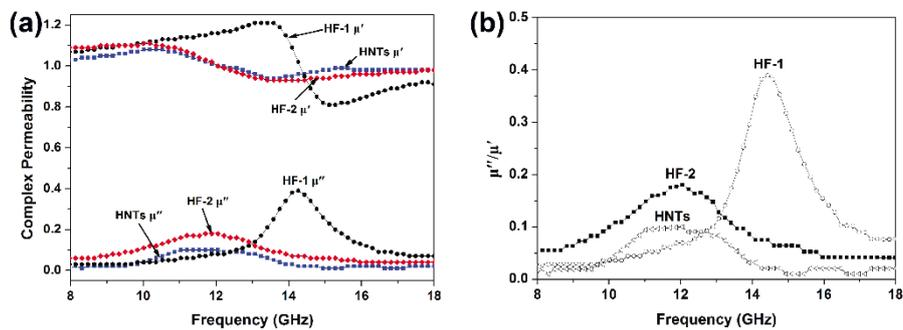
**Fig. S4** Frequency dependence of (a) relative complex permeability, and (b) magnetic loss tangents of natural halloysite (HNTs), MnFe<sub>2</sub>O<sub>4</sub>/halloysite nanotubular encapsulates (HF-1), and MnFe<sub>2</sub>O<sub>4</sub>/halloysite nanocomposites (HF-2).
