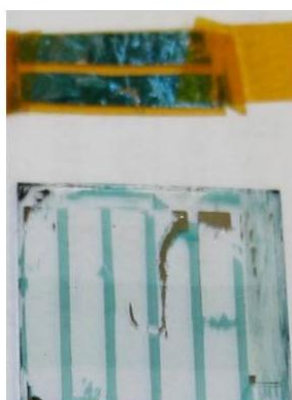
Figure S4. Digital camera images showing the effect of post-annealing treatment on the interface between the active layer and the metal cathode.
