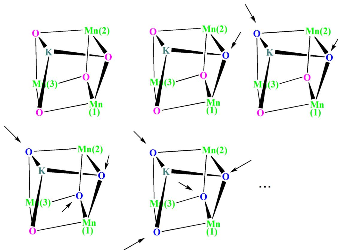
Fig. S6 Different motifs are formed by adding  $\text{H}_2^{18}\text{O}$  to nanolayered Mn-K oxide. Each motif may differ DRIFT peak in Mn-O-Mn area. Arrows show isotopic oxygen in the structure.
