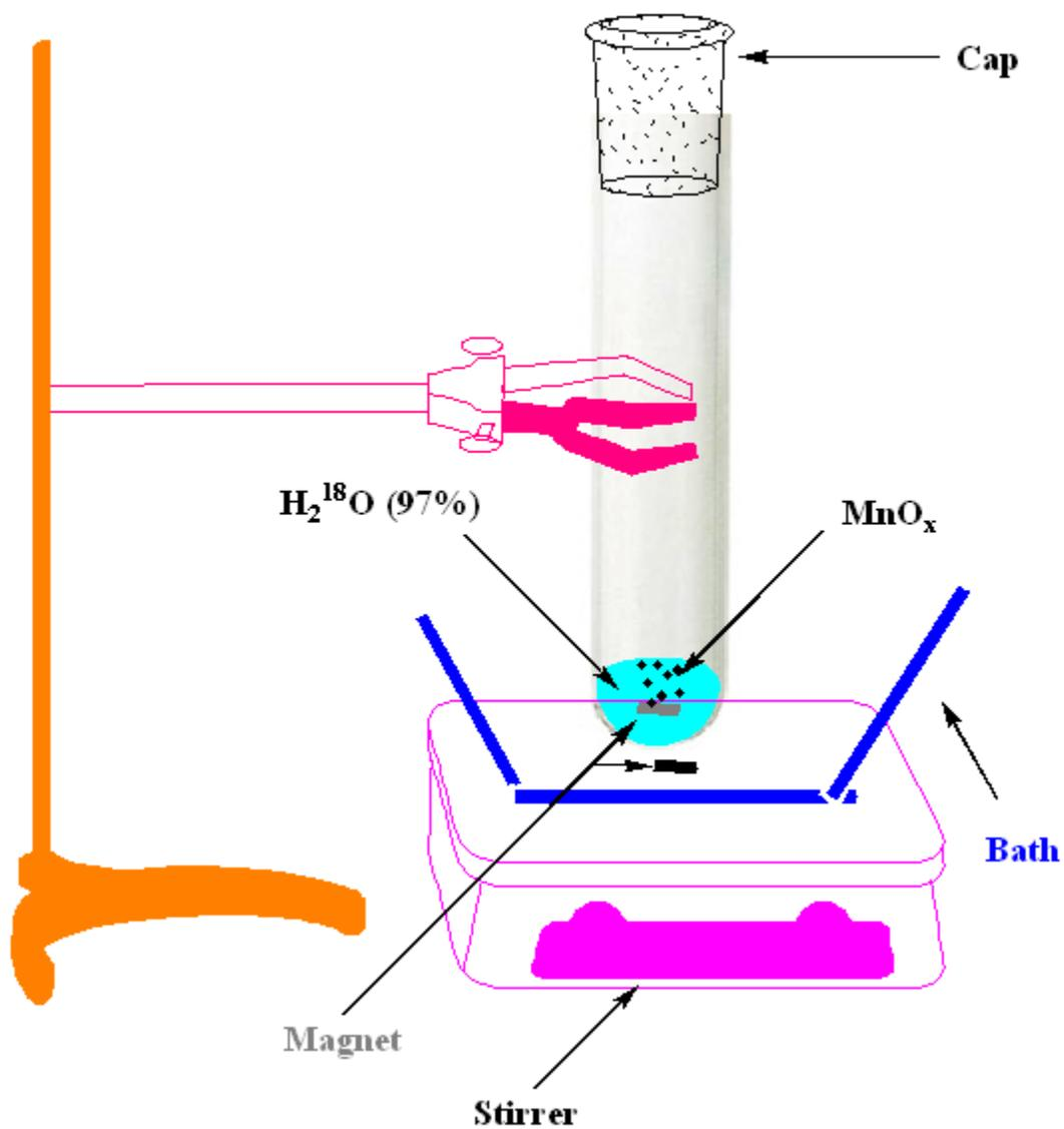
Scheme S1 Set up for finding the rate of exchange for  $\mu\text{-O}$  on the surface of layered Mn oxide by diffuse reflectance infrared Fourier transform spectroscopy.
