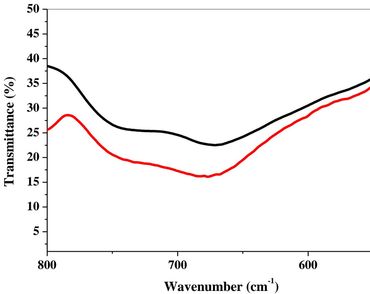
Fig. S11 DRIFT spectra of reference compound (black) and reference compound after 900 s (red).
