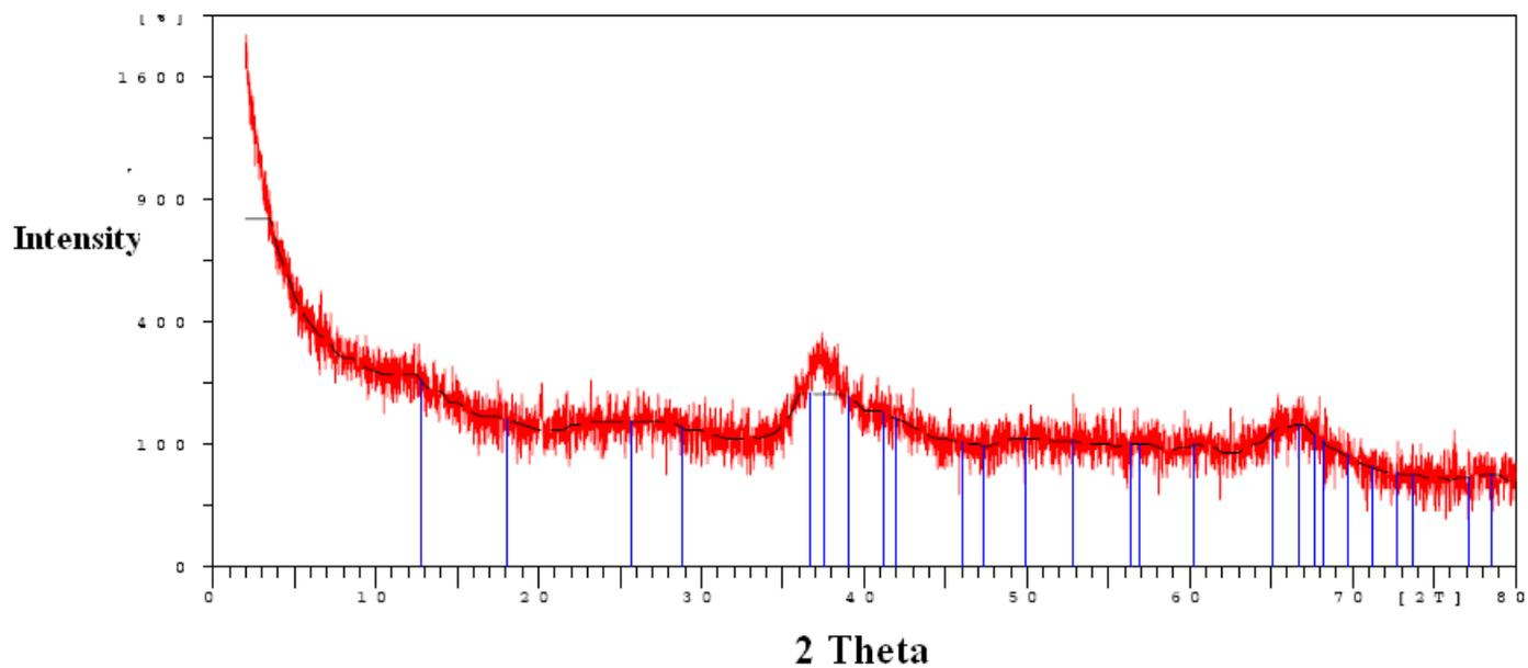
Fig. S4 XRD of nanolayered Mn-K prepared at 200 °C.
