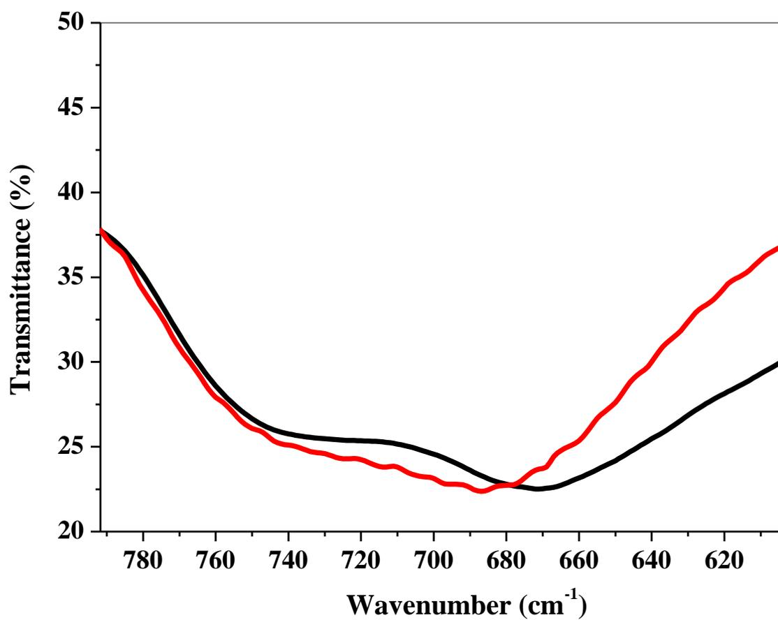
Fig. S13 DRIFT spectra of reference compound (black) and reference compound after 2 days (red).
