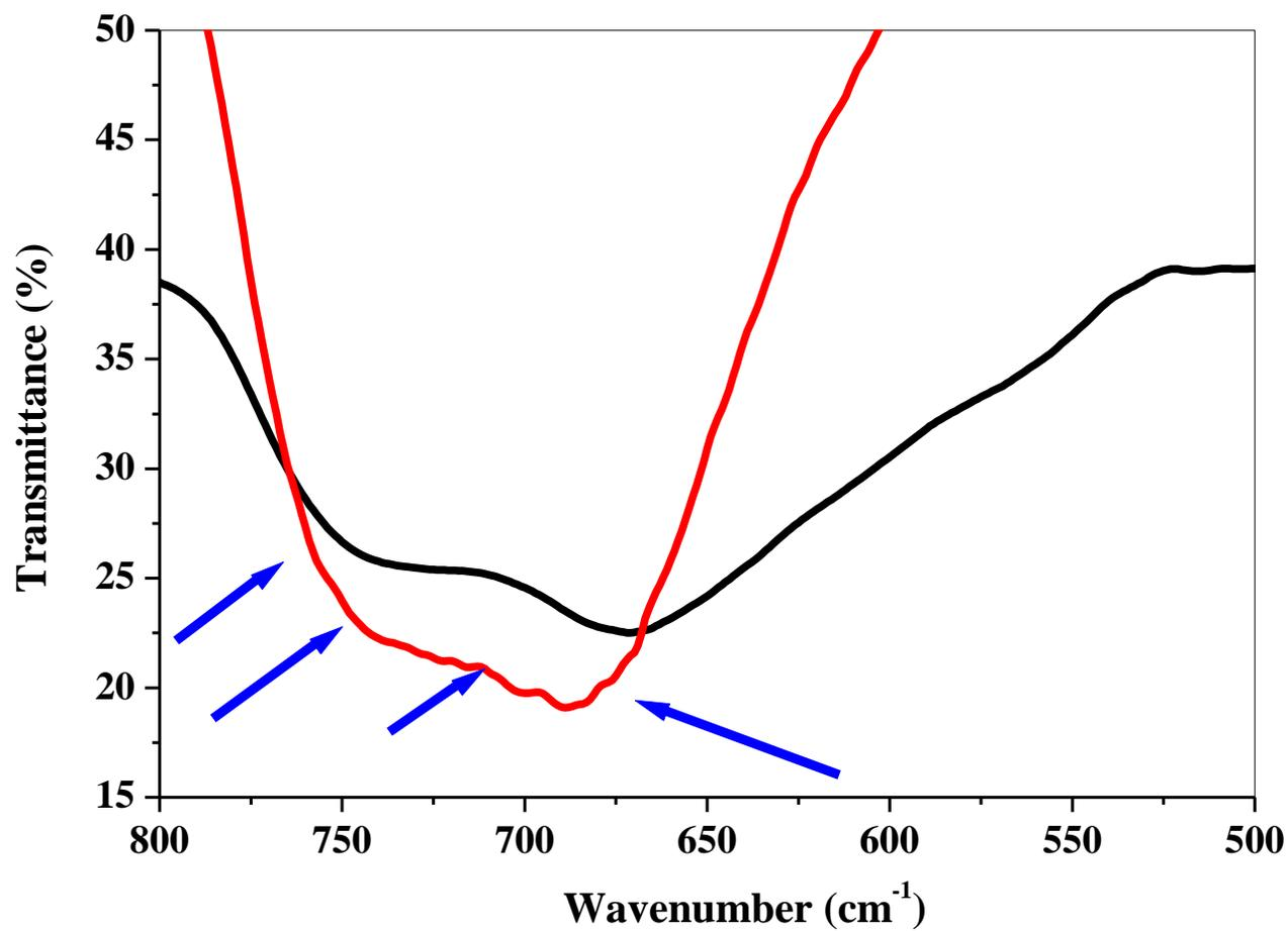
Fig. S14 DRIFT spectra of reference compound (black) and reference compound after one week (red). Blue arrows show new peaks related to <sup>18</sup>O in Mn oxide.
