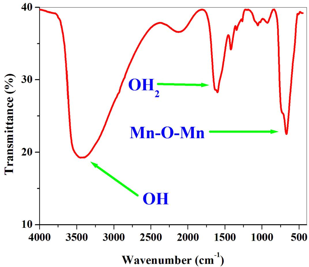
Fig. S3 Diffuse reflectance infrared Fourier transform spectrum of nanolayered Mn-K.
