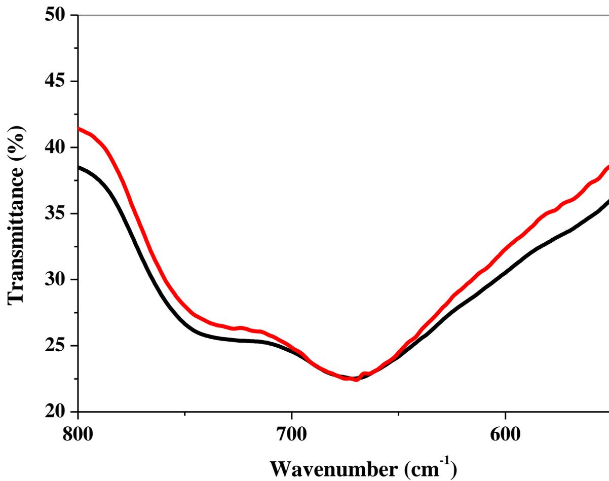
Fig. S7 DRIFT spectra of reference compound (black) and reference compound after 30 s (red).
