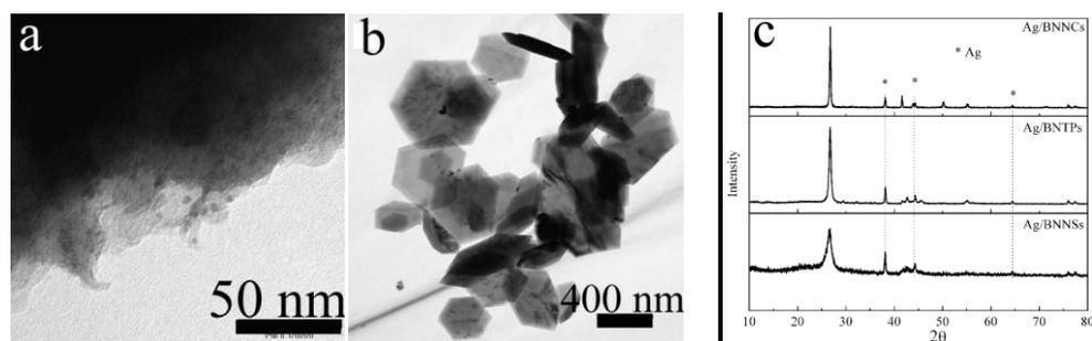
Fig. SI 4. TEM images of Ag/BNNs (a) and Ag/BNNCs (b), the XRD patterns of three types of Ag/BN nanomaterials were shown in (c), the Ag was marked by “\*”, it is basically consistent with the JCPDs No. 04-0783. The Ag nanoparticles was estimated to be around 5~20 nm for the Ag/BNNs and Ag/BNNCs.
