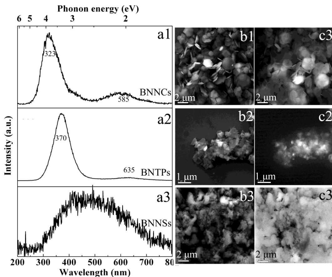
Fig. SI 3. The Cathodoluminescence of BNNCs (a1)<sup>12a</sup>, BNTPs (a2) and BNNSs (a3) collected at room temperature. The corresponding SEM and CL images are shown in middle (b1, b2 and b3) and right panel (c1, c2 and c3).
