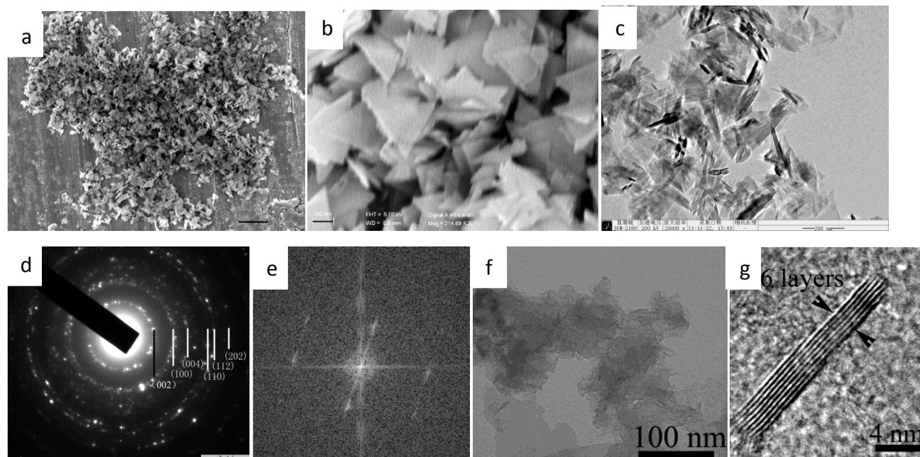
Fig. SI 1. SEM(a,b), TEM (c,f) and HRTEM(g) images of BNTPs(a-e) and BNNSs (f,h), the SAED pattern (d) corresponds to (c), the pattern was indexed base on the *h*-BN phase, the FFT pattern (e) was got from the HRTEM images in Fig. 3d. The thinness of agglomerated ultrathin BNNSs was mainly in the range of 1~6 nm (f), a typical BNNSs constituted with 6~8 layers (g).
