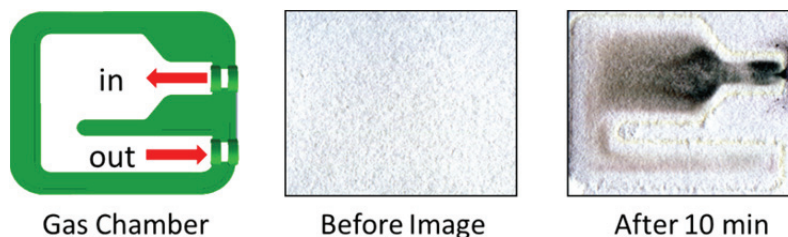
Fig. S3. Experiment with rectangular flow chamber shows non laminar entrance flow. Area near the inlet port changed the most, but very small color change is observed near the exhaust port. The membrane was exposed to saturated vapor of 2,4-DNT.
