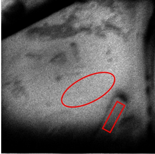
Figure: The SIMS total ion image of PAA at week 3 with displayed regions of interest for open polymer areas (oval) and HAp features (rectangle). Individual mass spectra from each region of interest were summed and are compared to reference spectra.
