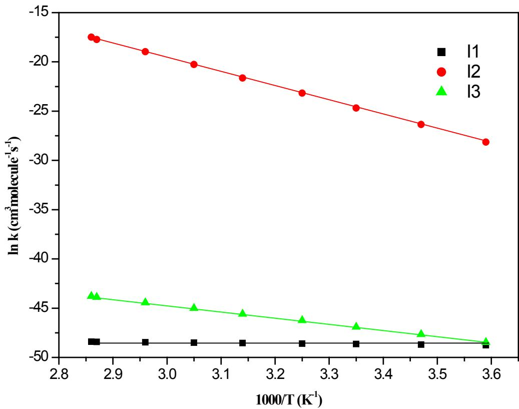
**Figure S2:** Arrhenius plot of the rate constant calculated for the intermediates, I1, I2 and I3 over the temperature range of 278-350 K
