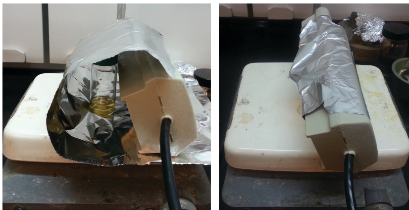
Fig. S1. TEC reaction setup. Reaction was carried out using handheld UV lamp at room temperature.
