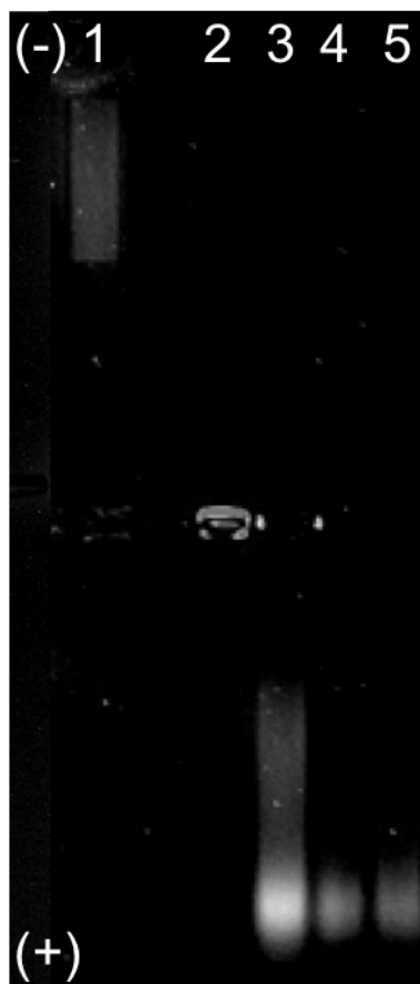
Fig. SI 2. Electrophoresis of UCNP before and after functionalization. Lanes correspond to samples (1) UCNP-APTMS, (2) UCNP-APTMS-BSA, (3) UCNP-APTMS-Dex, (4) UCNP-APTMS-BSA/Dex, and (5) UCNP-APTMS-BSA/Dex-Strv5.0. UCNP were revealed under 405 nm excitation wavelength.
