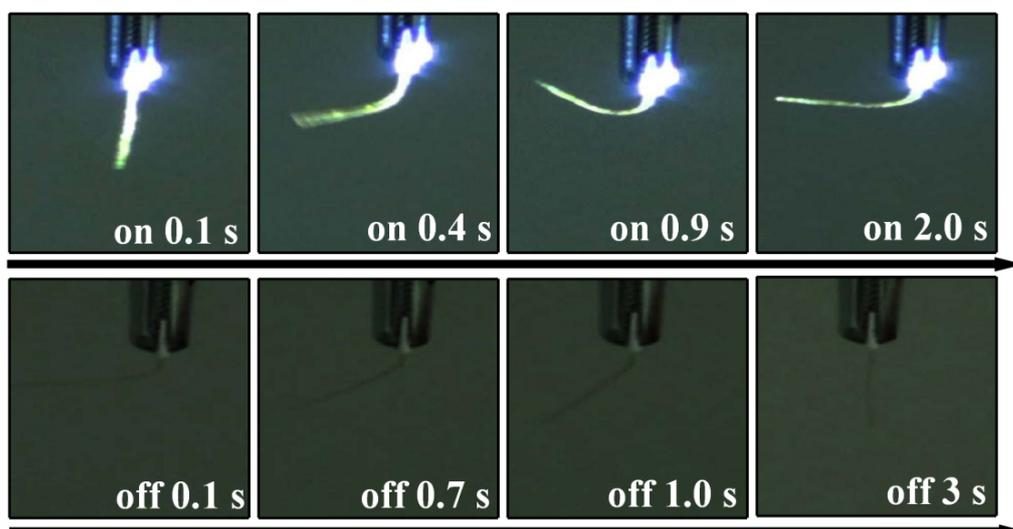
**Figure S6.** The process of reversible bending of SFA actuators (2 mm × 12 mm × 16 μm) alternate controlled with UV light (365 nm, 70 mW/cm<sup>2</sup>).
