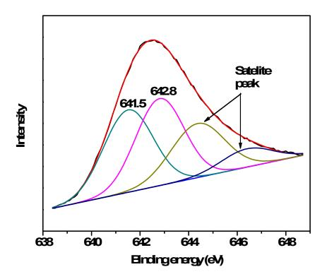
Fig. S1 XPS of Mn  $2p_{3/2}$  of MnOx-ST used catalyst after three recycles
