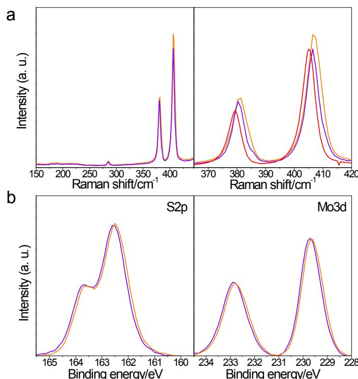
**Figure S1.** (a, b) Raman and (b, c) XPS spectra corresponding to films deposited from aqueous dispersions of MoS<sub>2</sub> stabilized with Brij700 (orange trace) and PVP (purple trace). (a) General and (b) detailed Raman spectra; (c) high resolution S2p core level XPS spectra; (d) high resolution Mo3d core level XPS spectra.
