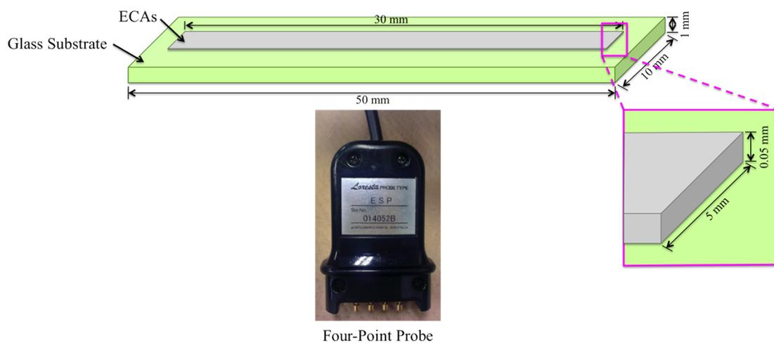
Figure S1 Diagram of tested sample for bulk resistivity and the four-point probe
