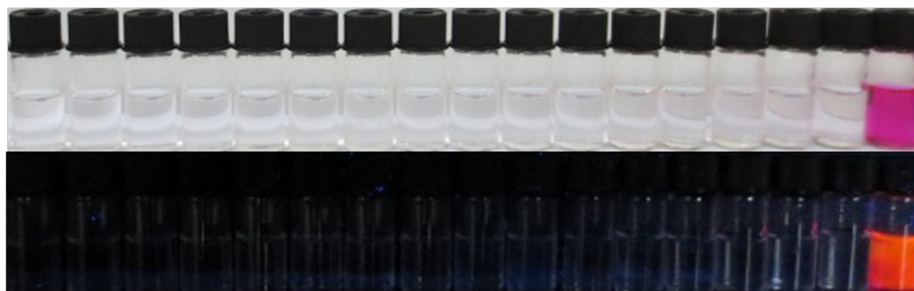
Fig. S9 Pictures of 3c as a selective naked-eye probe (top) and the visual fluorescence emissions by using a UV lamp (365 nm) (bottom) for Fe 3+ . From the left to right: blank, Ag + , Na + , K + , Ca 2+ , Cd 2+ , Mg 2+ , Co 2+ , Mn 2+ , Cu 2+ , Al 3+ , Zn 2+ , Ni 2+ , Fe 2+ , Hg 2+ , Cr 3+ and Fe 3+ ions.
