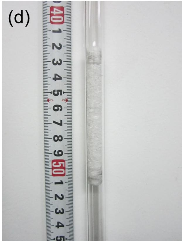
**Fig. S9** Photos of the quartz tube: (a) before and (b) after the blank tube test with dry mixed gas, and (c) before and (d) after the blank tube test with wet mixed gas.
