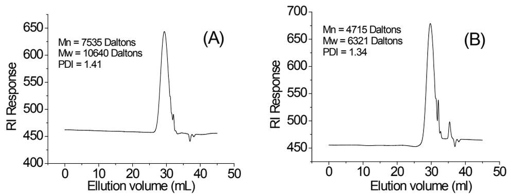
**Fig. S4** GPC traces of (A) SPAES-30 and (B) SPAES -40
