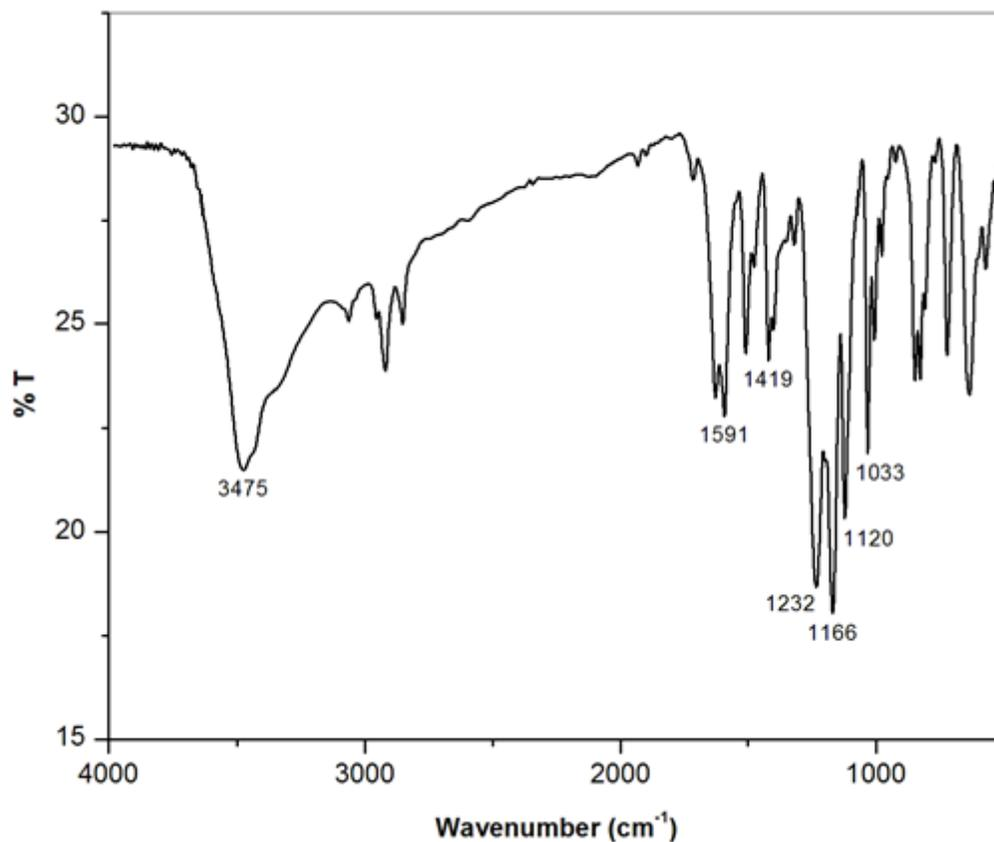
**Fig. S2** FTIR spectrum of azo based diol.
