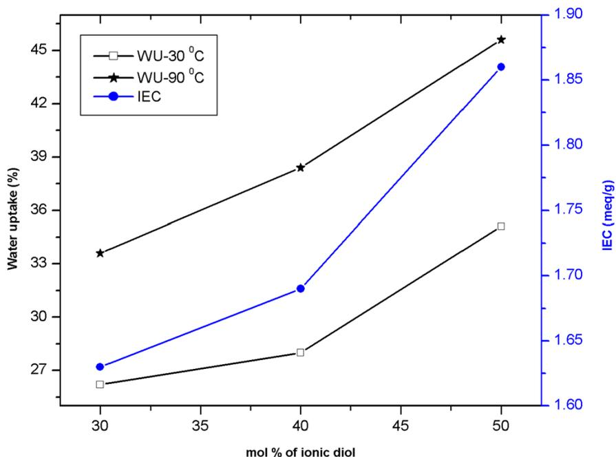
**Fig. S3** Water uptake and ion-exchange capacity of the SPAES membranes.
