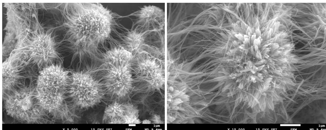
**Fig. S8** SEM images the catalyst after the test of the catalytic ability cycle
