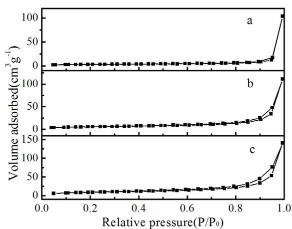
**Fig. S1** Nitrogen adsorption-desorption isotherms of the sample S1 (a), S2 (b), and S3 (c) obtained at different concentration of precursors.
