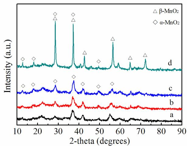
**Fig. S3** The XRD patterns of samples obtained at different time: (a) 15 min, (b) 2h, (c) 6h, (d) 10h.
