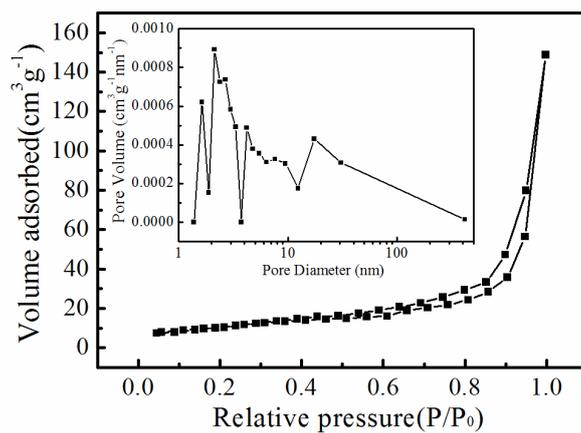
**Fig. S9** Nitrogen adsorption-desorption isotherms and pore size distribution (inset) of the catalyst after the test of the catalytic ability cycle
