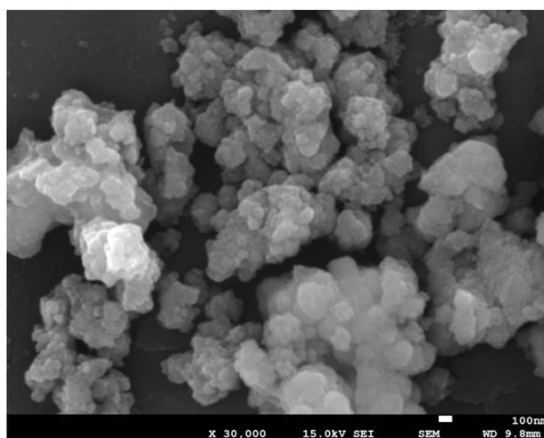
**Fig. S5** SEM images of commercial MnO<sub>2</sub>
