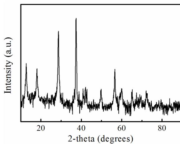
**Fig. S7** XRD pattern of the catalyst after the test of the catalytic ability cycle
