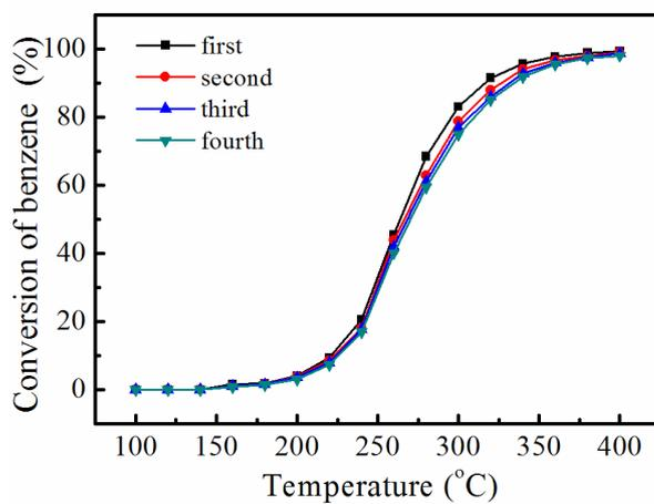
**Fig. S10** The catalytic ability cycle of S3 in the catalytic oxidation of benzene
