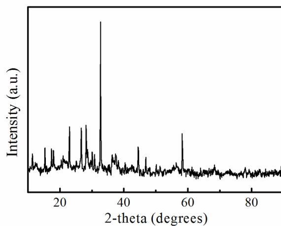
**Fig. S6** XRD pattern of commercial MnO<sub>2</sub>
