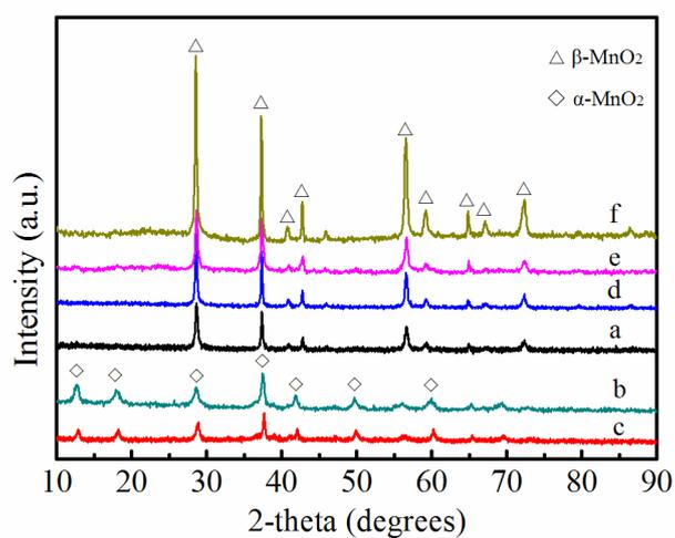
**Fig. S2** The XRD patterns of samples obtained at different concentration of precursors.
