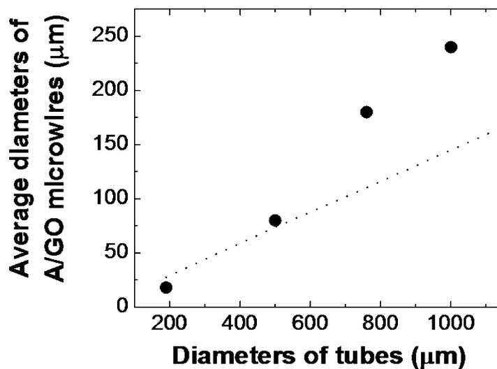
Fig. S4. A/GO microwire diameter as a function of the extrusion tube inner diameter. Dotted line is the calculated diameter assuming only radial contraction when water is evaporated.
