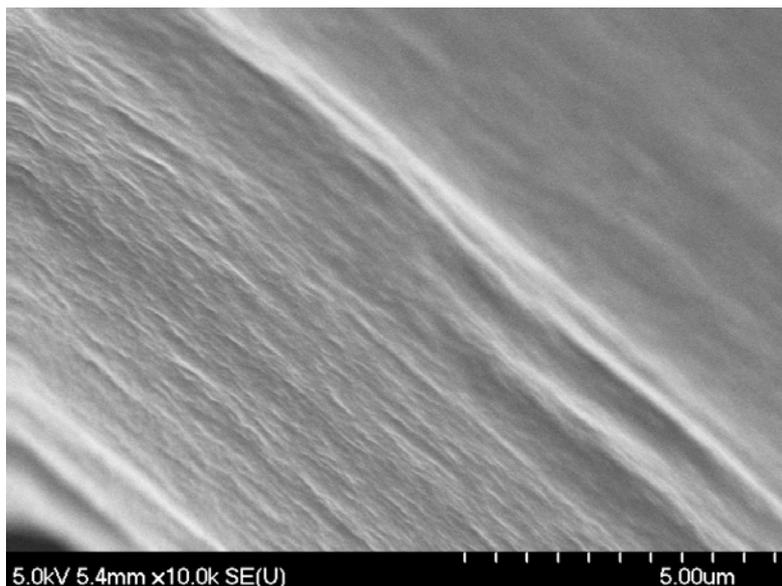
Fig. S5. SEM image of A/rGO composite wires prepared from A/GO hydrogel containing 0.1 wt.% GO.
