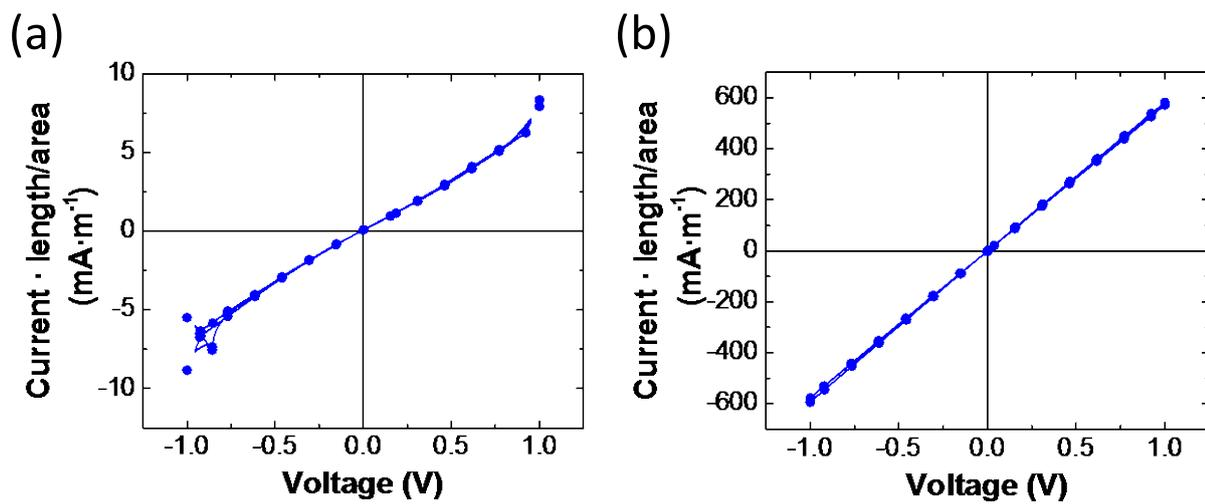
Fig. S8. I-V curves of A/rGO microwire after the thermal treatment at (a) 200 °C and (b) 300 °C.
