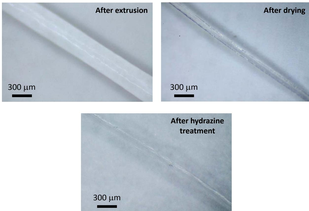
Fig. S3. Optical images of GO-free agarose wires. The agarose content is 2 wt.% before drying.
