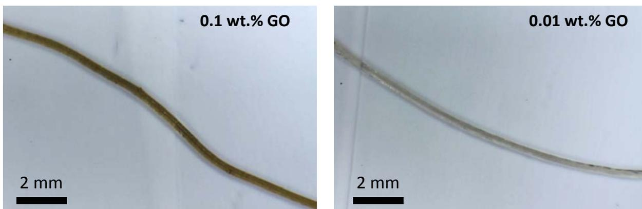
Fig. S2. Low magnification optical images of A/GO composite wires of the samples (a) and (b) in Fig. 2.
