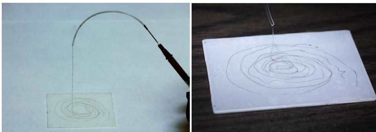
Fig. S1. Extrusion of the GO-loaded agarose gel.
