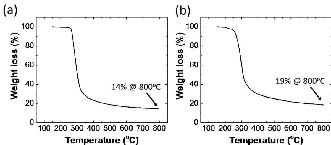
Fig. S6. TGA curves of (a) agarose and (b) dried A/rGO (2 wt.% of agarose and 0.1 wt.% of graphene oxide before drying of 97.9wt.% of water). The TGA measurement was conducted in air at a heating rate of 10 °C/min. The residual weight is 5% higher in (b) than (a), which is because of the thermally stable rGO (weight percent of rGO in the dried A/rGO composite is 0.1 wt.%/2.1 wt.%  $\approx$  5 wt.%).
