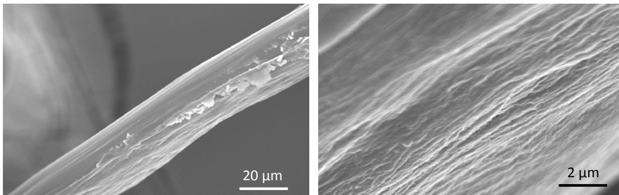
Fig. S7. SEM images of A/rGO composite wires after 400 °C heat treatment.
