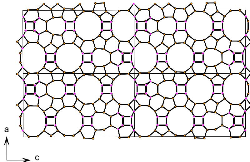
**Figure S6:** Projection along the *a*-axis of IM-17 in space group *Amm2*.
