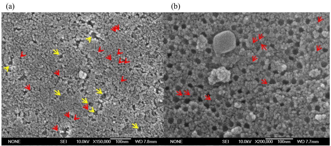
Figure S2: FE-SEM images of mesoporous silicas templated by TEOS/F127/PEO-*b*-PCL = 3/0.9/0.7 using spin-coating process (a) and EISA process (b).
