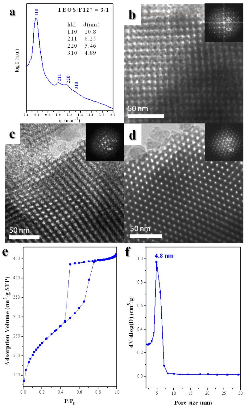
**Figure S1.** (a) SAXS pattern, (b–d) TEM images viewed from (b) [100], (c) [110], and (d) [111] (insets: corresponding FFT), (e)  $N_2$  adsorption/desorption isotherm, and (f) pore size distribution curve of the *bcc* mesoporous silica templated by F127 at a TEOS-to-F127 ratio of 3:1.
