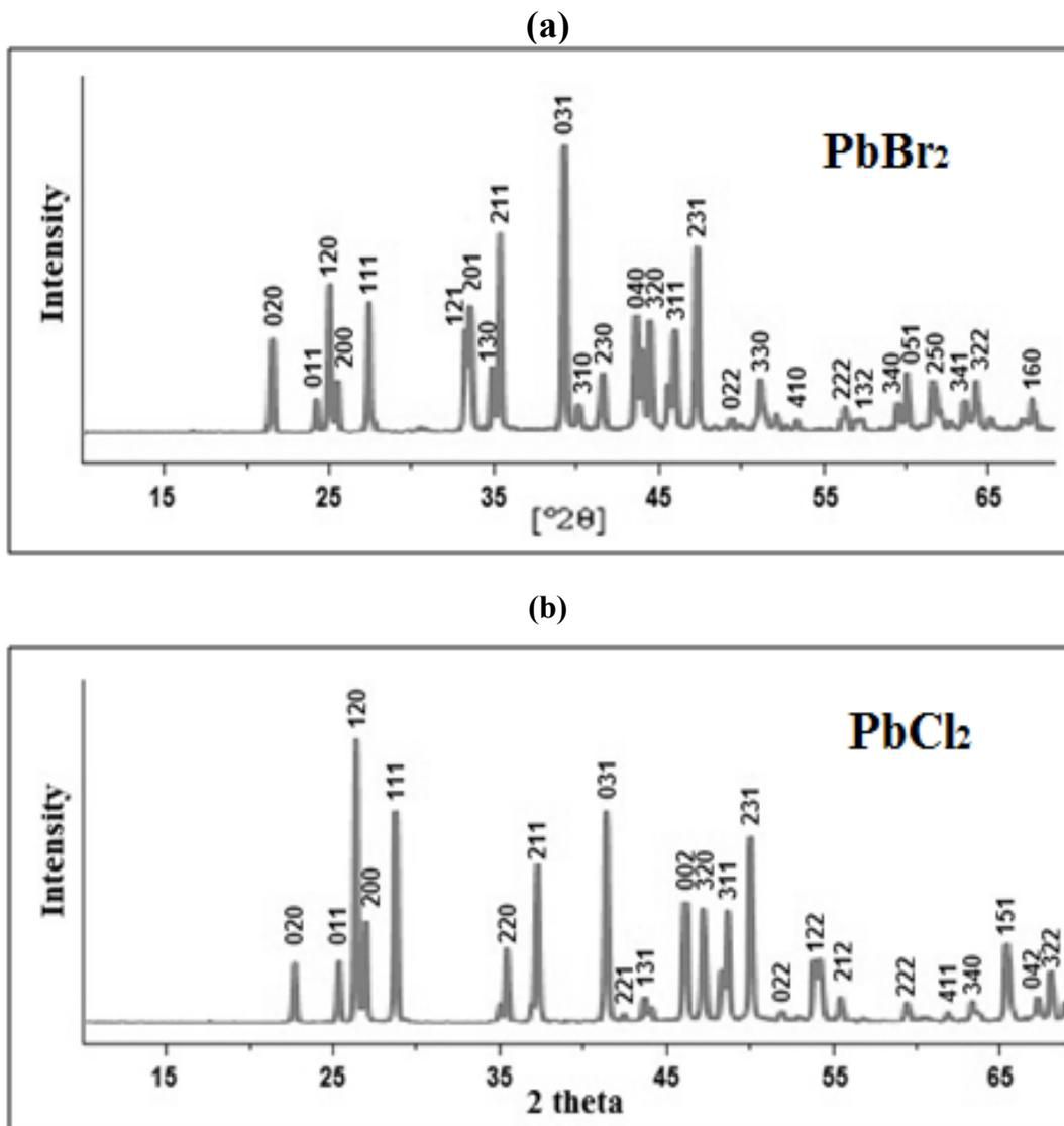
**Fig. S6** XRD patterns of (a) PbBr<sub>2</sub> and (b) PbCl<sub>2</sub> nanoparticles prepared by thermolysis of compounds **1** and **2** in oleic acid at 180 °C under air atmosphere for 2 h, respectively.
