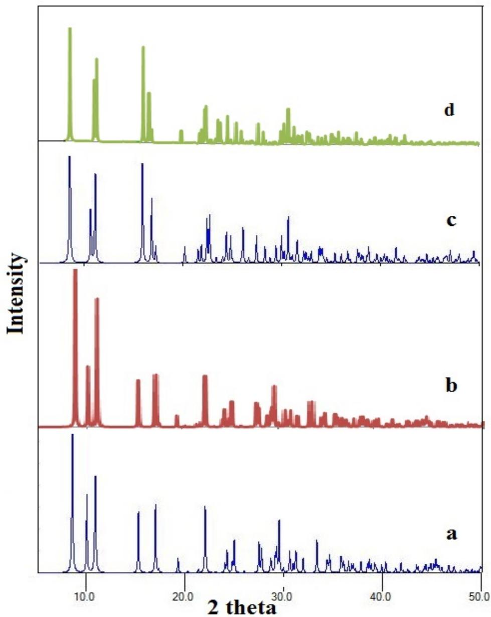
**Fig. S3** The XRD patterns of (a) simulated from single crystal X-ray data of compound **1**, (b) bulk materials obtained by solid state anion-replacement of compound **2** with 2 mmol KBr, (c) simulated from single crystal X-ray data of compound **2**, (d) bulk materials obtained by solid state anion-replacement of compound **1** with 2 mmol KCl.
