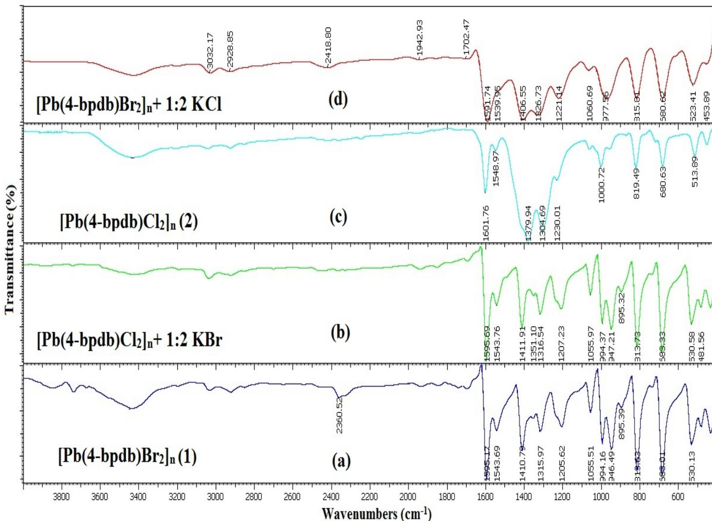
**Fig. S4** IR spectra of (a) compound **1**, (b) bulk materials obtained by solid state anion-replacement of compound **2** by grinding with 2 mmol KBr, (c) compound **2** and (d) bulk materials obtained by solid state anion-replacement of compound **1** by grinding with 2 mmol KCl.
