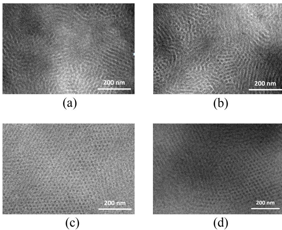
**Fig. SI-6** TEM image of  $V_{36}H_{77}V_{36}$  (a, b) and  $V_{30}H_{123}V_{30}$  (c, d).
