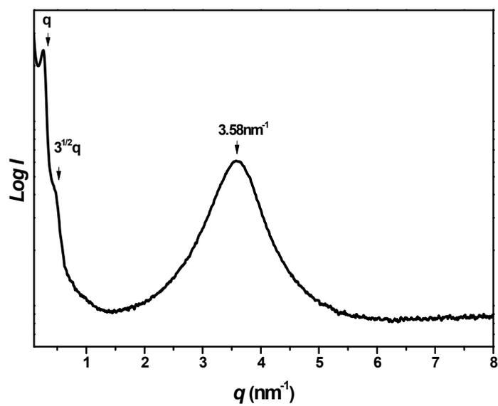
**Fig. SI-7** XRD profile of a typical triblock copolymer of  $V_{30}H_{123}V_{30}$  recorded at 160 °C.
