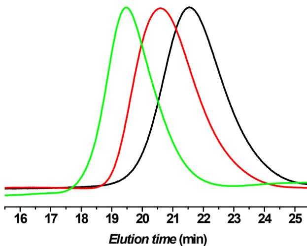
**Fig. SI-2** GPC traces of difunctional macroinitiator Cl-PHCS-Cl. From right to left, the traces correspond to the samples with the  $M_{n, GPC}$  of 11600, 18000, and 33200  $g\ mol^{-1}$  calibrated with polystyrene standards.
