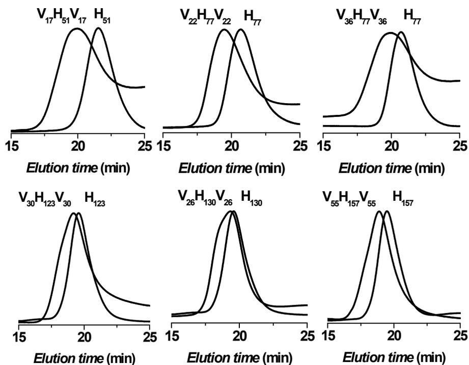
**Fig. SI-3** GPC traces of triblocks of P4VP-*b*-PHCS-*b*-P4VP (V<sub>X</sub>H<sub>Y</sub>V<sub>X</sub>) and the corresponding macroinitiator Cl-PHCS-Cl. THF was used as the eluent at a flow rate of 1.0 ml min<sup>-1</sup>.
