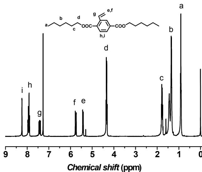
**Fig. SI-1**  $^1H$  NMR spectrum of 2,5-di(*n*-hexogycarbonyl)styrene (HCS) monomer (Sample in  $CDCl_3$ , 400 MHz).
