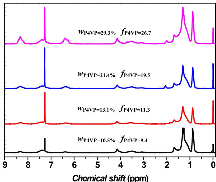
**Fig. SI-4**  $^1\text{H}$  NMR spectra of the P4VP-*b*-PHCS-*b*-P4VP triblock copolymers with various P4VP contents. (samples in  $\text{CDCl}_3$ , 400 MHz).
