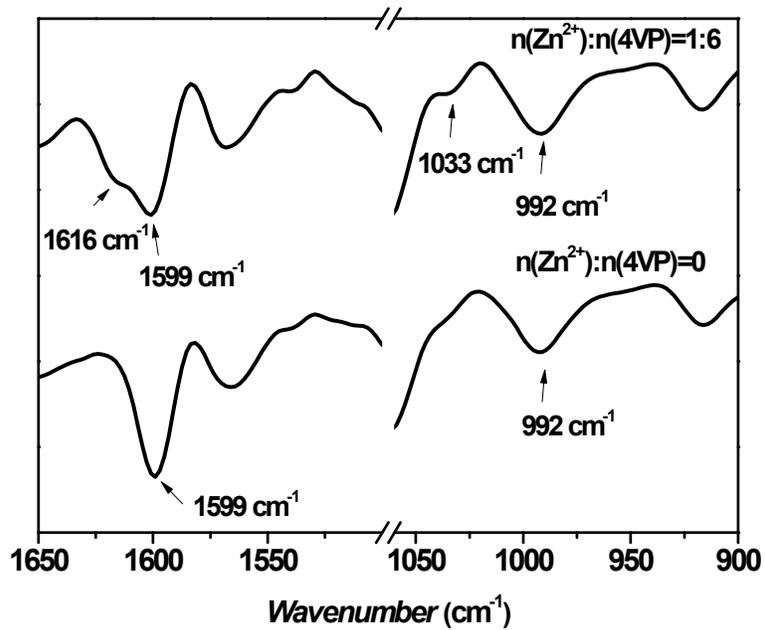
**Fig. SI-8** FTIR spectra recorded in the region 1630-1500  $\text{cm}^{-1}$  and 1060-900  $\text{cm}^{-1}$  for the pure triblock  $\text{V}_{30}\text{H}_{123}\text{V}_{30}$  and the triblock complexed with zinc perchlorate.  $n(\text{Zn}^{2+}):n(4\text{VP})$  is the molar ratio of  $\text{Zn}^{2+}$  to the repeating unit of 4VP.
