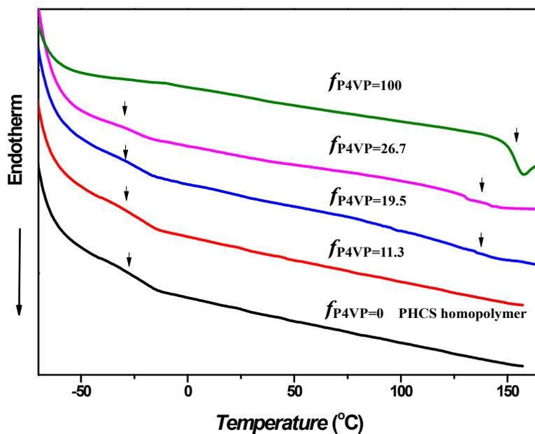
**Fig. SI-5** DSC curves of the triblock copolymers with variable  $f_{\text{P4VP}}$  recorded during the second heating scan at a rate of  $40\text{ }^\circ\text{C min}^{-1}$ .
