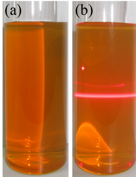
Figure S3: The light brown transparent solution of \text{Fe}(\text{OH})_3 (a) and its Tyndall effect (b).
