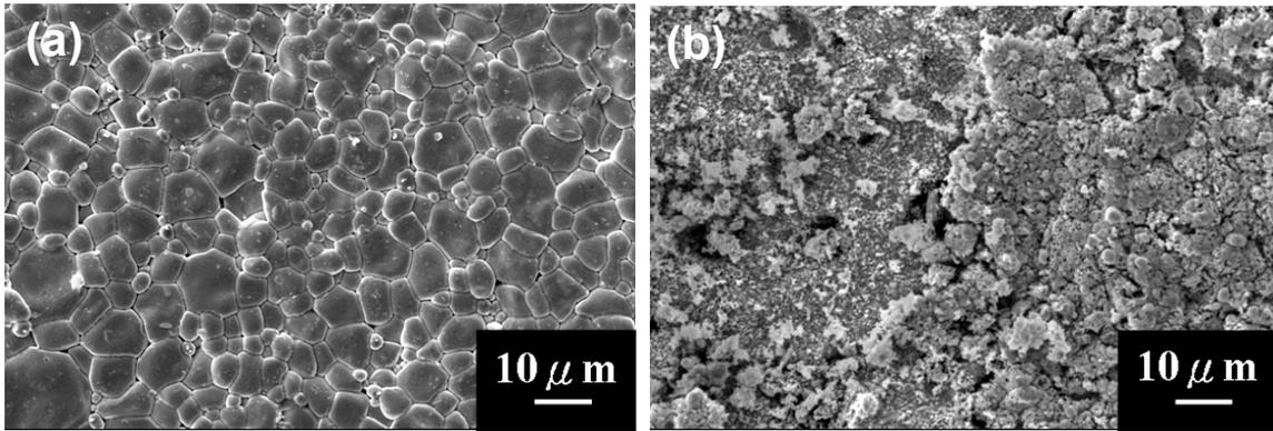
**Fig. S2** SEM photos of BFO only electrolyte (a) before and (b) after the fuel cell operated at 700°C.
