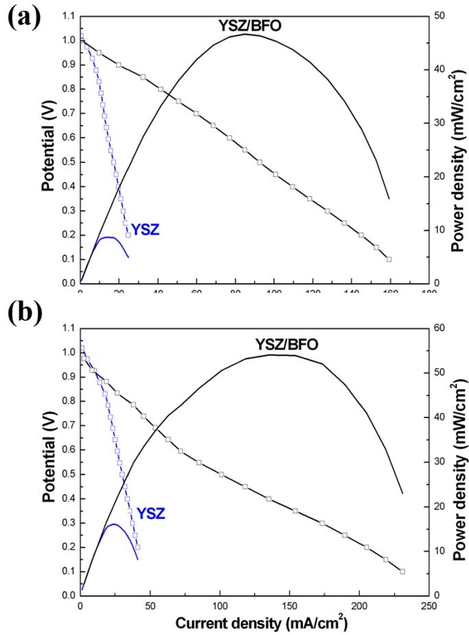
**Fig. S3** Comparison of fuel cells performance with YSZ/BFO (103μm/38μm) electrolytes or YSZ (98μm) electrolyte at (a) 650°C and (b) 700°C operating temperature.
