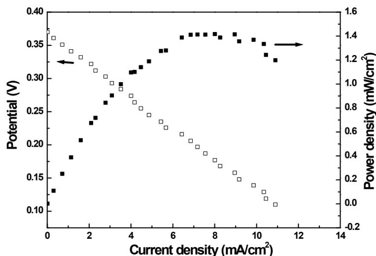
**Fig. S1** Fuel cell performance using BFO only electrolyte at 700°C.
