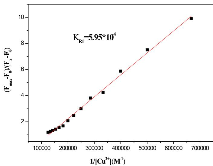
**Fig. S4.** Determination of binding constant of **MP** with  $\text{Cu}^{2+}$  using Benesi-Hildebrand equation
