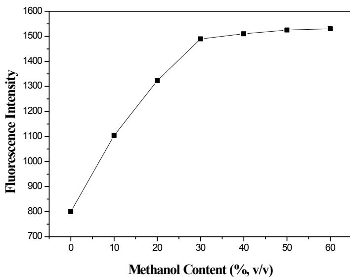
**Fig. S1.** Effect of the methanol content on the fluorescence intensity of **MP** (10  $\mu\text{M}$ ) with the presence of  $\text{Cu}^{2+}$  (10  $\mu\text{M}$ ) for 20 min,  $\lambda_{\text{ex}} = 535 \text{ nm}$ .
