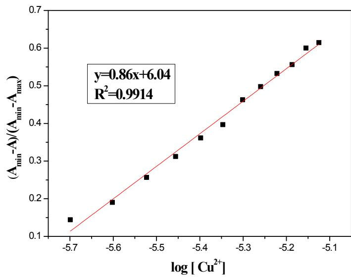
**Fig. S3.** The plot of absorption intensity at 552 nm of **MP** vs.  $\text{Cu}^{2+}$  concentrations.
