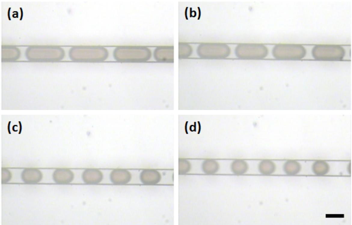
**Fig. S4** An example images of generated microdroplets by dyed water using pneumatic pumps. In this experiments, positive pressure is increased 0 kPa to 10 kPa ((a) ~ (d)) against fixed negative pressure at -40 kPa. 5 The generated microdroplets maintain uniformity under stable fixed pressure conditions. Scale bar: 100 $\mu$ m.
