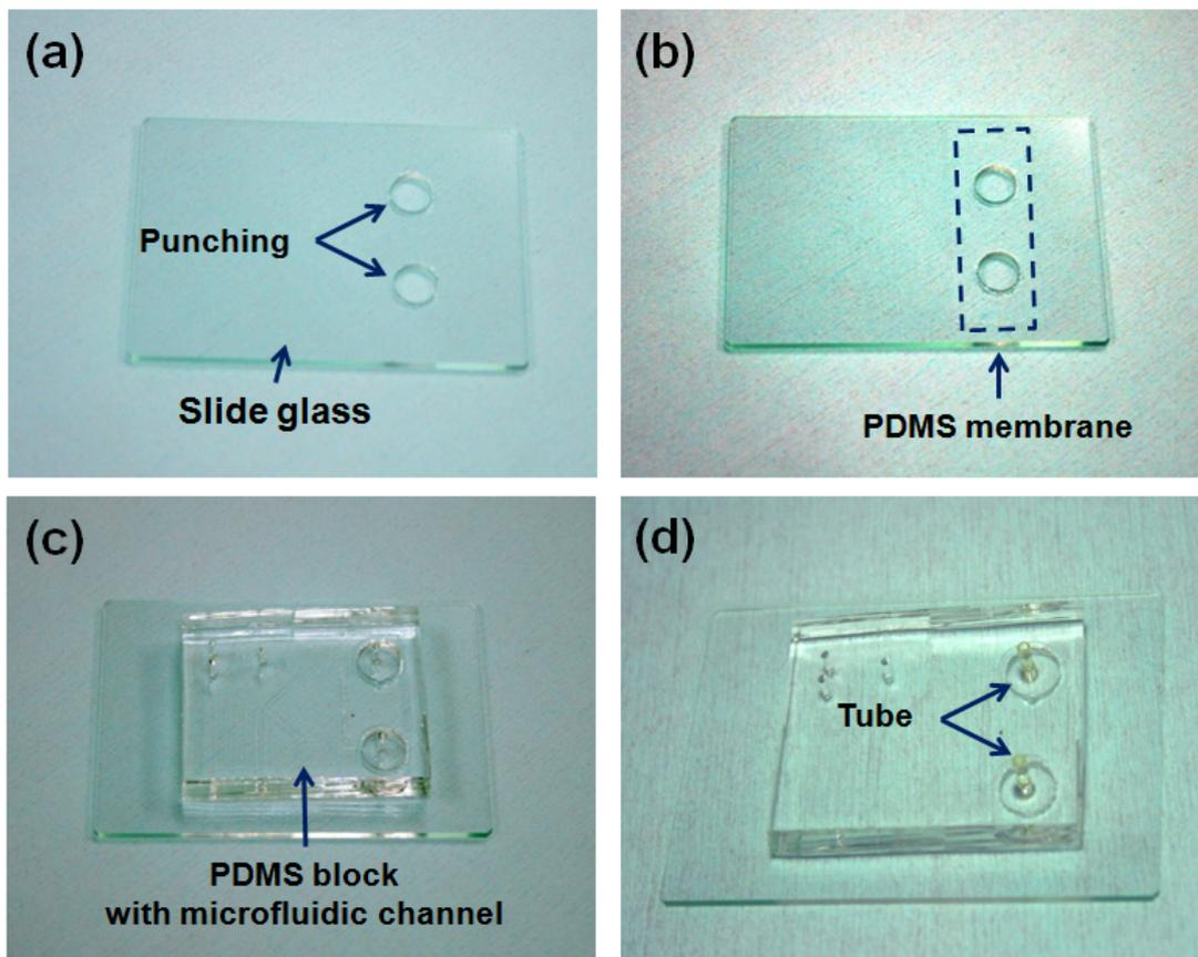
**5 Fig. S2** Assemble process of microfluidic chip for integrated pneumatic micro-pumps. Firstly, (a) glass substrate was punched with 8 mm hole using milling machine. Secondly, (b) Flexible polydimethylsiloxane (PDMS) membrane was attached on bottom side of slide glass. Thirdly, (c) PDMS block containing structured microfluidic channel was bonded on upside of slide glass after oxygen plasma treatment. Finally, (d) polyurethane tube was inserted into PDMS block.
