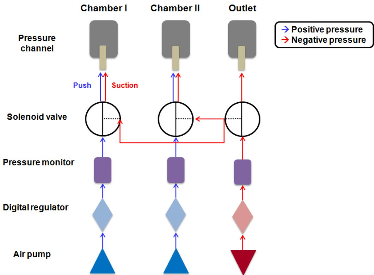
**Fig. S3** Schematic of a pressure control system for the PDMS diaphragm actuations of the pumps. The applied positive and negative pressures are controlled with air pumps, digital regulators (ITV series, SMC Co., Noblesville, IN, USA), pressure monitors and a solenoid valve (LHD series, Lee Company, Westbrook, CT, USA). The digital regulators (i.e., electro-pneumatic and electronic vacuum regulators) control positive and negative (0.1 kPa per 0.01 V).
