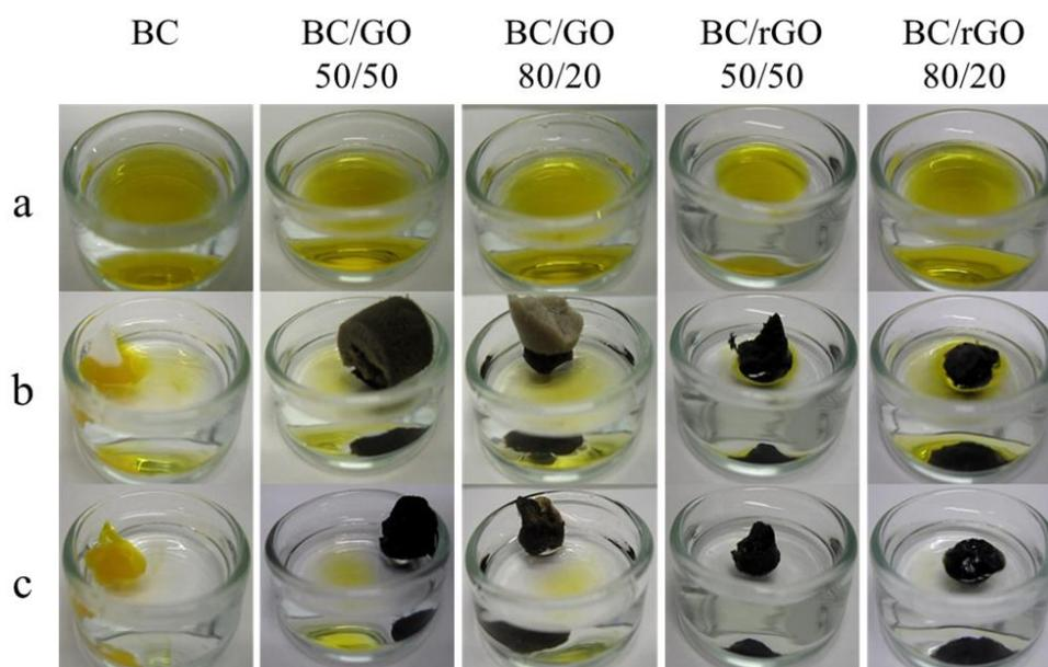
**Figure S4.** Representative images showing the absorption of cyclohexane (dyed with Sudan I) from water surface with a: dyed cyclohexane on water surface in petri dishes; b: placement of aerogel onto the surface of the mixture and begin of the absorption; c: end of the absorption.
