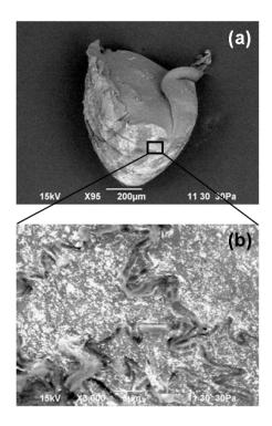
**Figure S1**: Backscattered electron SEM images showing (a) the cross section of the stem of the dried mushroom-like structure, and (b) a detail at high magnification of its surface.
