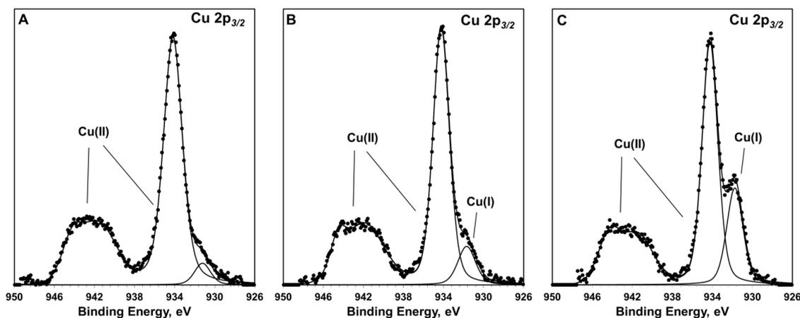
**Fig. S3** XPS spectra of the Cu 2p<sub>3/2</sub> peak collected at 90° take-off angle for 10 min (A), 20° take-off angle for 10 min (B) and 90° take-off angle for 2h10min (C) respectively. Samples were immersed in CuSO<sub>4</sub> (200 ppb), cooled with liquid N<sub>2</sub> both during the introduction into the spectrometer and in the analysis chamber during the 10 min experiment. The spectra have had the background subtracted and Cu(II) and Cu(I) contributions fitted.
