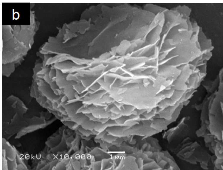
Fig. S1 SEM images of the as-synthesized MCH template.
