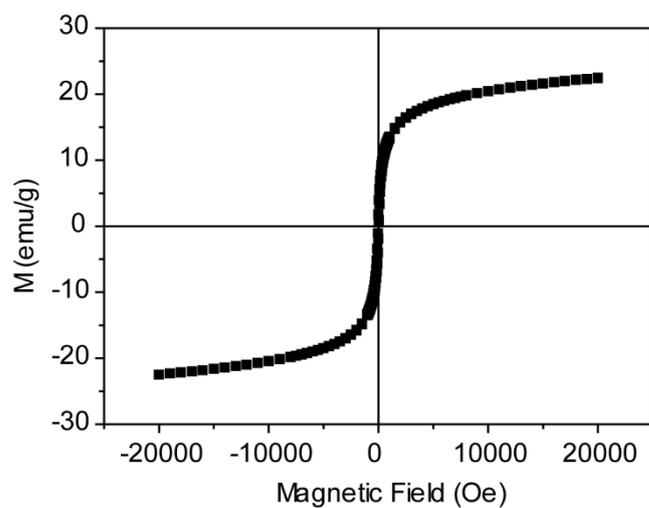
Figure S3. The magnetic hysteresis loops at 300 K of  $\text{Fe}_3\text{O}_4$ -Silica-Yolk-Shell.
