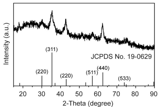
Figure S2. XRD pattern of  $\text{Fe}_3\text{O}_4$  Silica Yolk-Shell structure.
