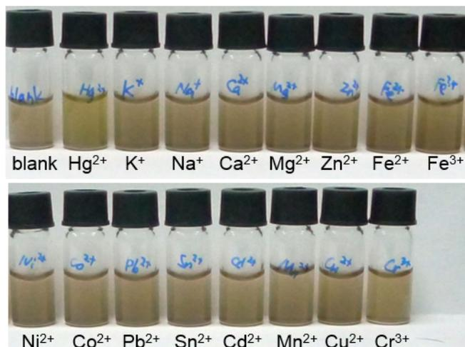
Figure S9. Color change of the aqueous solution of  $\text{Fe}_3\text{O}_4$ -YS-N719 in the presence of various representative metal ions.
