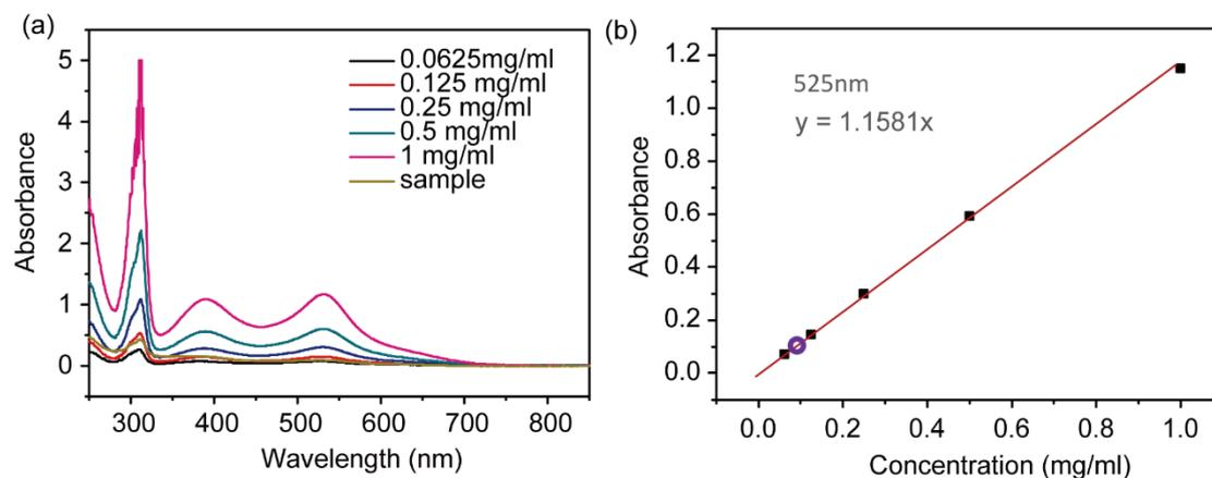
Figure S7. (a) UV-vis absorption spectra of N719 with different concentrations. (b) The absorbance at 530 nm as a function of N719 concentration. The N719 content on Fe<sub>3</sub>O<sub>4</sub>-YS-N719 was determined to be 5.3 wt%.
