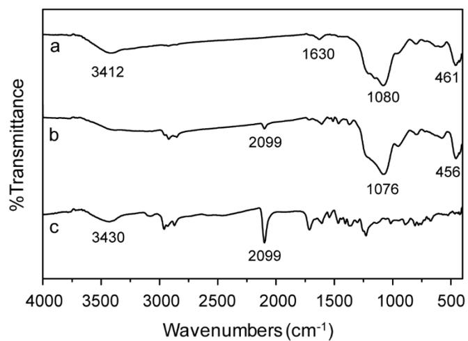
Figure S6. FTIR spectra of (a) Fe<sub>3</sub>O<sub>4</sub>-Silica-Yolk-Shell, (b) Fe<sub>3</sub>O<sub>4</sub>-YS-N719, (c) N719.
