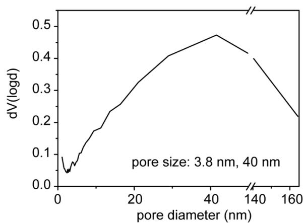
Figure S5. The corresponding Barrett-Joiner-Halenda (BJH) pore distributions of Fe<sub>3</sub>O<sub>4</sub>-Silica-Yolk-Shell.
