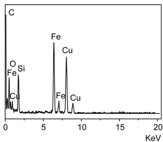
Figure S1. EDXA spectrum of  $\text{Fe}_3\text{O}_4$  Silica Yolk-Shell structure.
