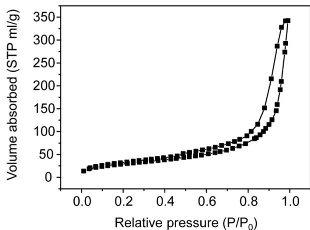
Figure S4. The nitrogen adsorption-desorption isotherms of Fe<sub>3</sub>O<sub>4</sub>-Silica-Yolk-Shell.
