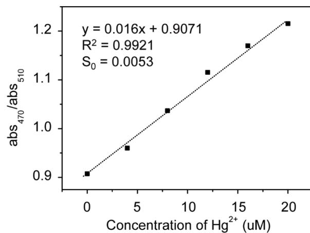
Figure S8. The sensitivity test of Fe<sub>3</sub>O<sub>4</sub>-YS-N719 using UV-vis absorption spectra. The detection limit of Hg<sup>2+</sup> was estimated to be 1 uM (200 ppb).
