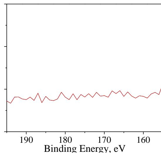
**Fig. S1** XPS spectra of Ag nanorods surface without MPBA-functionalization in S 2p and B 1s regions.
