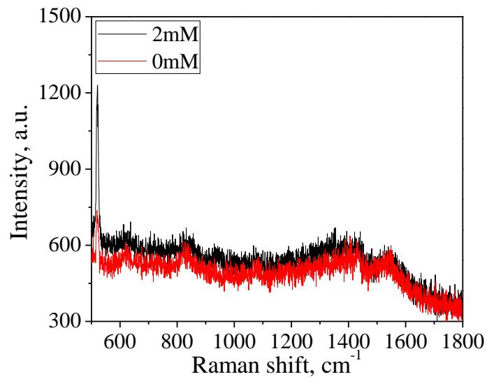
**Fig. S2** SERS spectra of 2 mM glucose and PBS buffer from Ag nanorod arrays without MPBA-functionalization. (The peak at ~520 cm<sup>-1</sup> was from Si on substrate)
