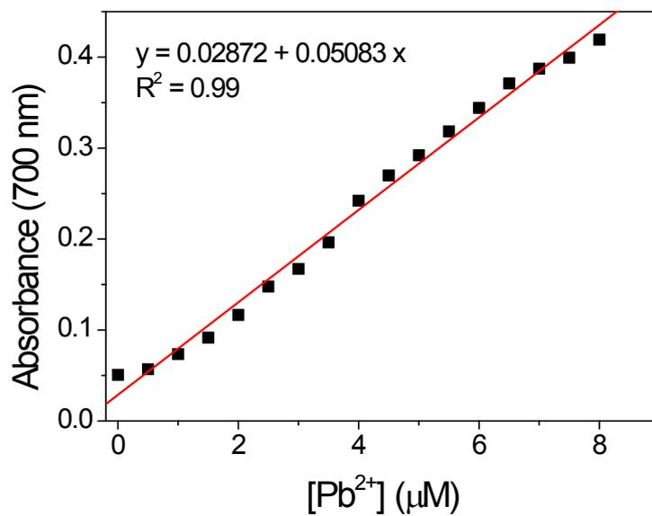
**Figure S1.** The calibration curve of TTA-AuNPs. The detection limit (DL) of HCS with HOCl was determined from the following equation:  $DL = K * S_b / S$ , where  $K = 3$ ;  $S_b$  is the standard deviation of the blank solution;  $S$  is the slope of the calibration curve.
