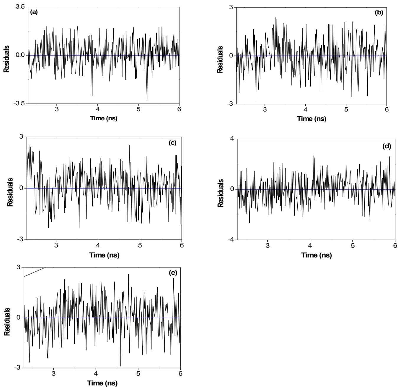
**Fig. S1:** Residual for the fitted fluorescence lifetime decay of (a) 7-DCCA in water, (b) in DTAB micellar medium, (c) in DTAB micellar medium in presence of 7 (M) urea, (d) in TTAB micellar medium and (e) in TTAB micellar medium in presence of 7 (M) urea.
