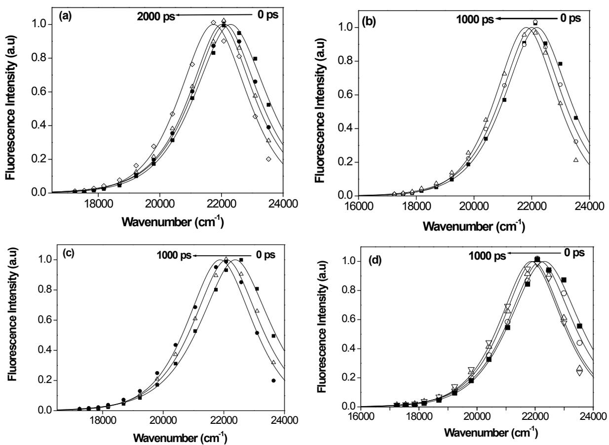
**Fig. S3:** Time resolved emission spectra (TRES) of 7-DCCA in (a) DTAB (b) TTAB (c) CTAB and (d) CDAB micellar media.
