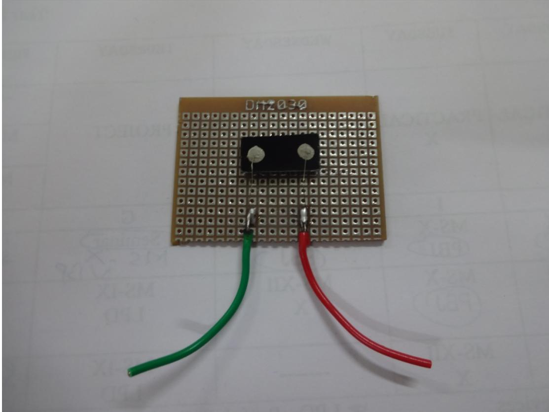
**Fig.2.** Photograph of CSA doped PPy/ $\alpha$ -Fe<sub>2</sub>O<sub>3</sub> hybrid sensor film .
