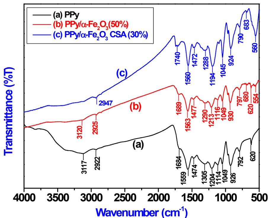
**Fig.3.** FTIR spectrum (a) PPy, (b) PPy/ $\alpha$ -Fe<sub>2</sub>O<sub>3</sub> (50%) and (c) 30% CSA doped PPy/ $\alpha$ -Fe<sub>2</sub>O<sub>3</sub> hybrid nanocomposite.
