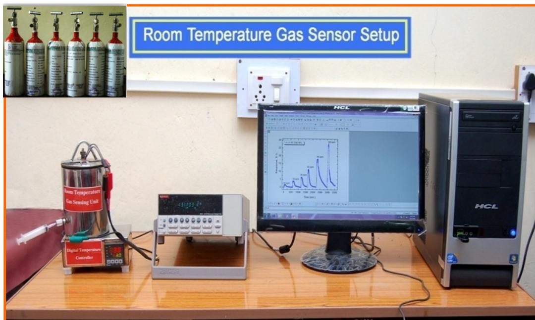
**Fig.1.** Experimental set up for room temperature gas sensing measurement.
