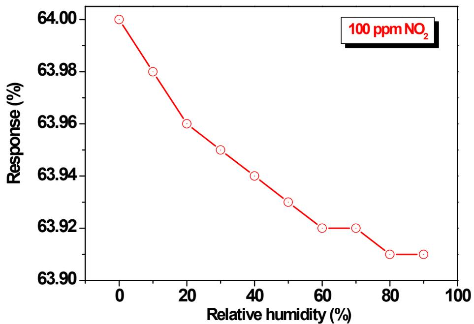
**Fig. 6 .** The variation of NO<sub>2</sub> response of CSA doped PPy/ $\alpha$ -Fe<sub>2</sub>O<sub>3</sub> film with 10-90% RH.
