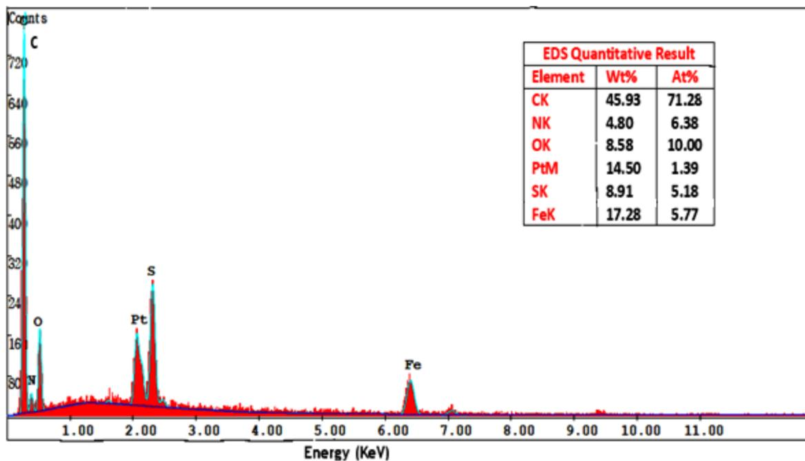
Fig.4. E-DAX spectrum of 30% CSA doped PPy/ $\alpha$ -Fe<sub>2</sub>O<sub>3</sub> hybrid nanocomposite.
