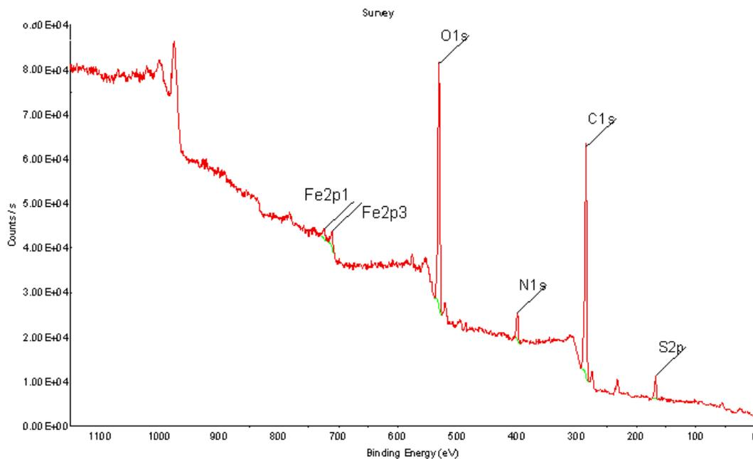
**Fig. 5.** XPS spectra of 30% CSA doped PPy/ $\alpha$ -Fe<sub>2</sub>O<sub>3</sub> hybrid nanocomposite.
