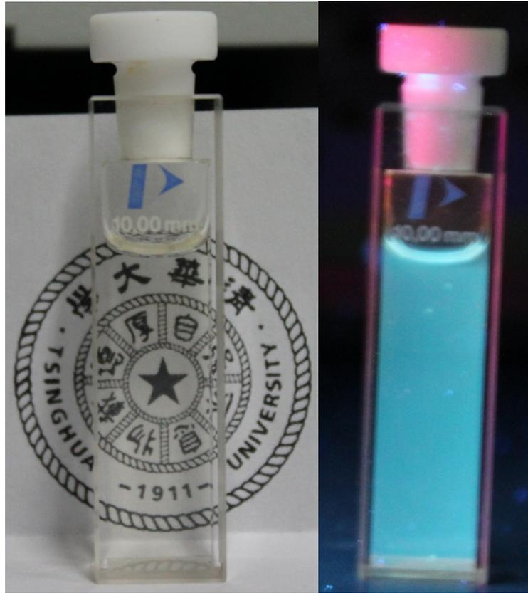
**Fig. S4** Optical images of **PEI-Mal** FONs water dispersion for more than one week (left bottle). The right bottle is the optical images of **PEI-Mal** FONs in water under UV lamp ( $\lambda = 365$  nm).
