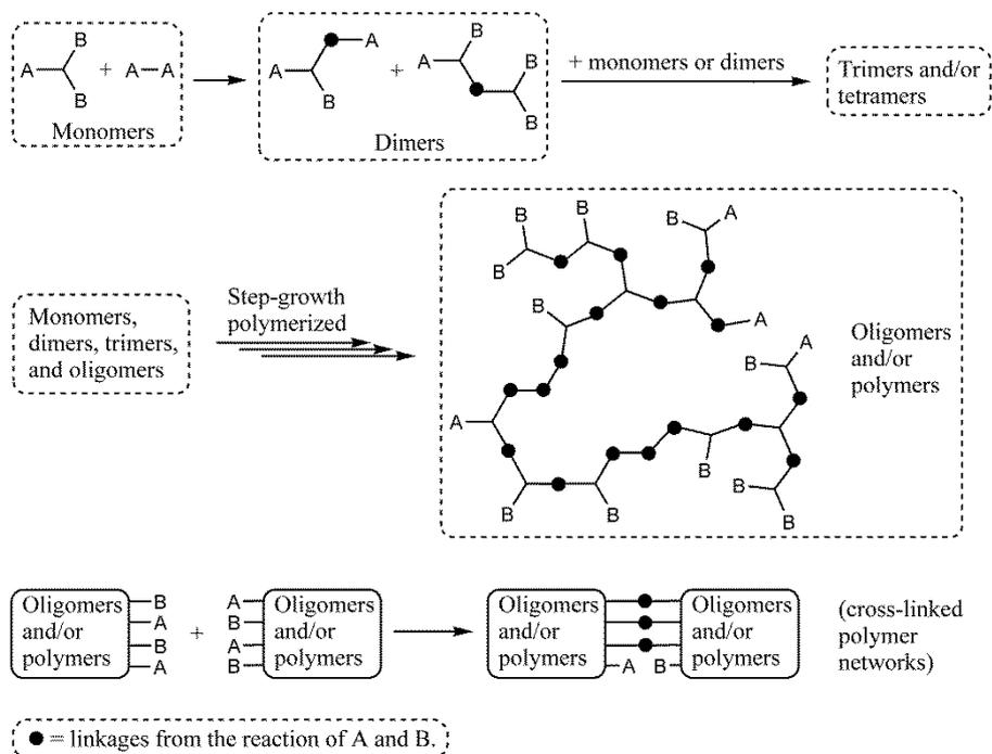
**Fig. S5.** Schematic representation of the synthesis of highly branched polymers from monomers AB<sub>2</sub> and A<sub>2</sub> (here, the functional group A and B are –COOH and epoxy groups, respectively, and the total amount of the –COOH groups is not greater than that of the epoxy groups in the feed).
