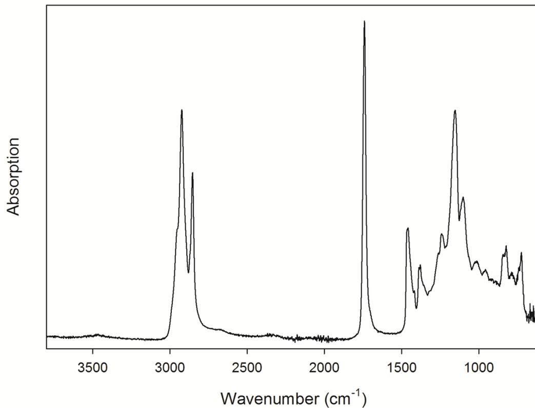
Fig. S1. FTIR spectrum of ESO obtained from Spectrum Chemical Manufacturing Corp. (New Brunswick, NJ).
