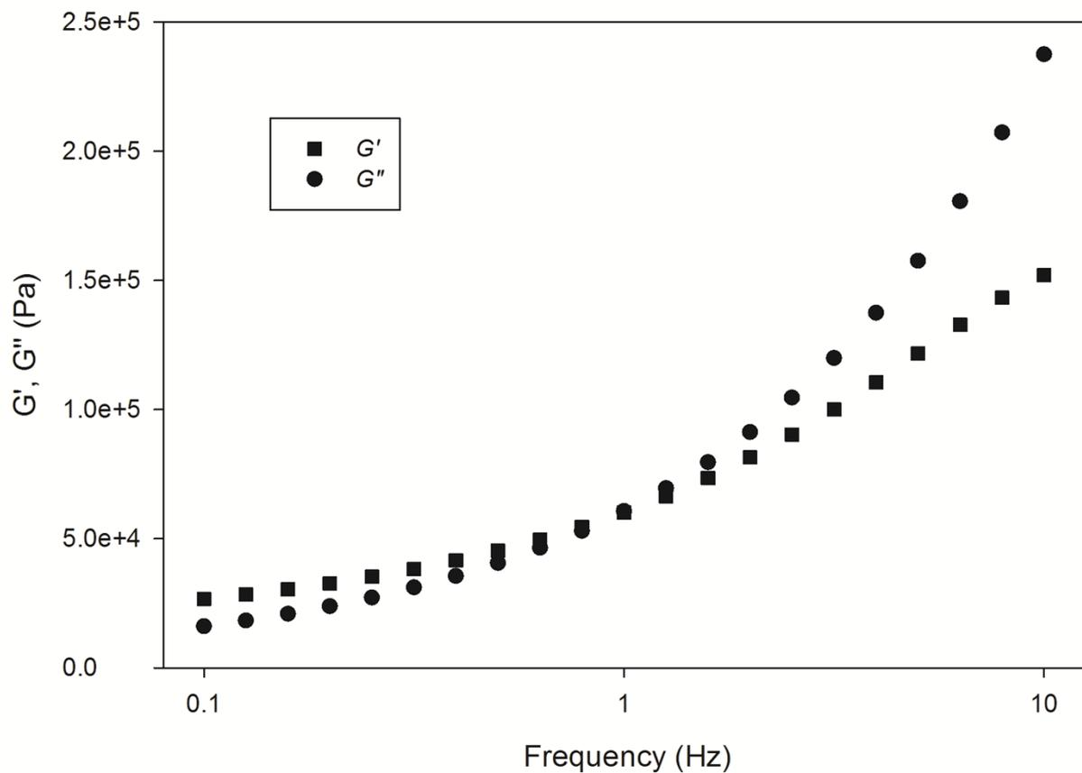
Fig. S6. Rheological profile ( $G'$  and  $G''$  vs frequency) for the EFAs-based PSA obtained from the copolymerization of the EFAs mixture and DA.
