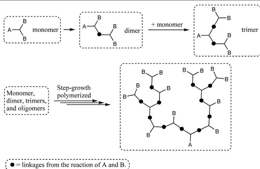
**Fig. S3.** Schematic representation of the synthesis of highly branched polymers from monomer  $AB_2$  (here, the functional group A and B are  $-\text{COOH}$  and epoxy groups, respectively).
