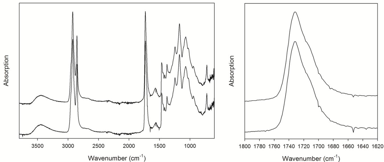
**Fig. S2.** FTIR spectra of the cured polymeric product by the polymerization of the EFAs mixture in the presence of AMC-2 (~1.6 wt% relative to the EFAs mixture) for a curing time of 15 min (left, bottom) and 75 min (left, top), respectively, and related close-up views (right) of the characteristic absorption signal due to the ester carbonyl stretching and the shoulder peak due to the -COOH carbonyl stretching which appeared on the right side of the ester carbonyl peak.
