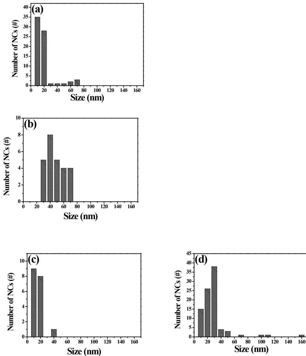
Figure S2. Size distribution of synthesized CZTS NCs prepared without complexing agent (a), with hydrazine (b), with Na<sub>3</sub>-citrate (c), and with Na<sub>2</sub>EDTA (d).
