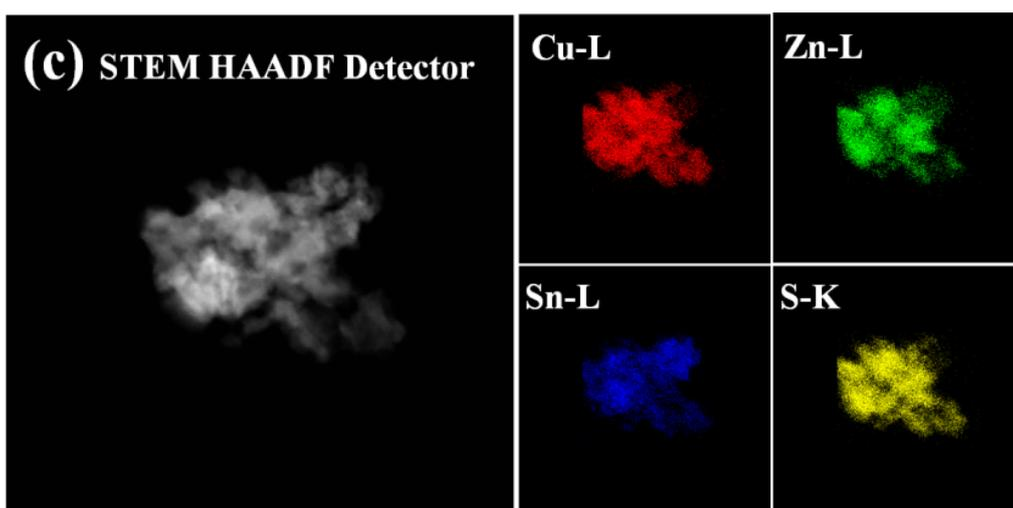
Figure S1. HAADF-STEM image and elemental mapping images of synthesized CZTS NCs prepared without complexing agent (a), with hydrazine (b), and with Na<sub>3</sub>-
