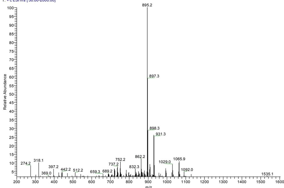
**Figure S5:** Mass of **RB-SP2-Cu<sup>2+</sup>** complex
