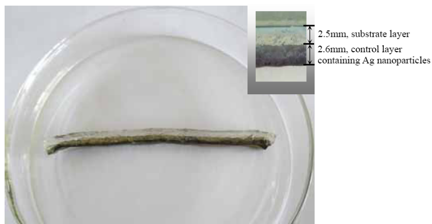
Fig. S1. Photograph of the two-layer shape memory reactor prepared. The small picture inserted is a partial amplified image
